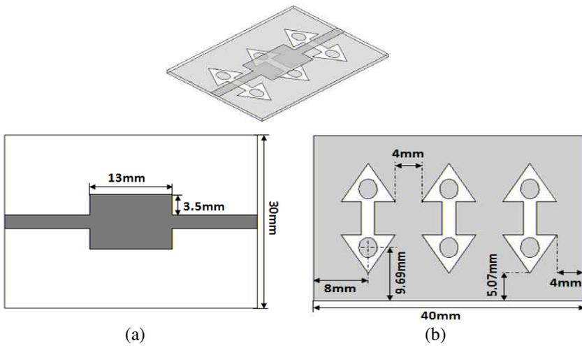
**Figure 2.** Schematic diagram of the prototype LPF (a) top layer and (b) bottom layer.
