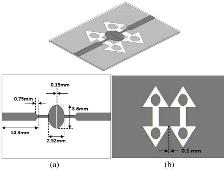
**Figure 9.** The geometry of the proposed BPF, (a) top view and (b) bottom view.
