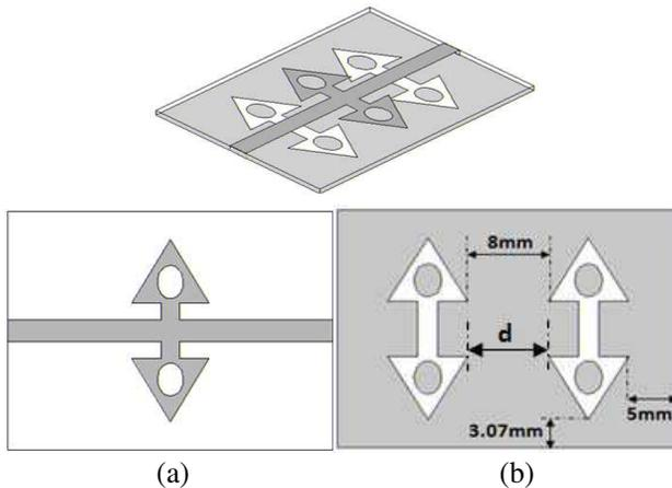
**Figure 4.** Schematic diagram of the multilayer LPF (a) top layer and (b) bottom layer.
