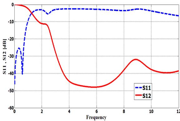
**Figure 3.**  $S$ -parameters results for the proposed LPF.
