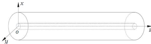
**Figure 1.** Cylindrical transverse electromagnetic wave inside the coaxial transmission line.
