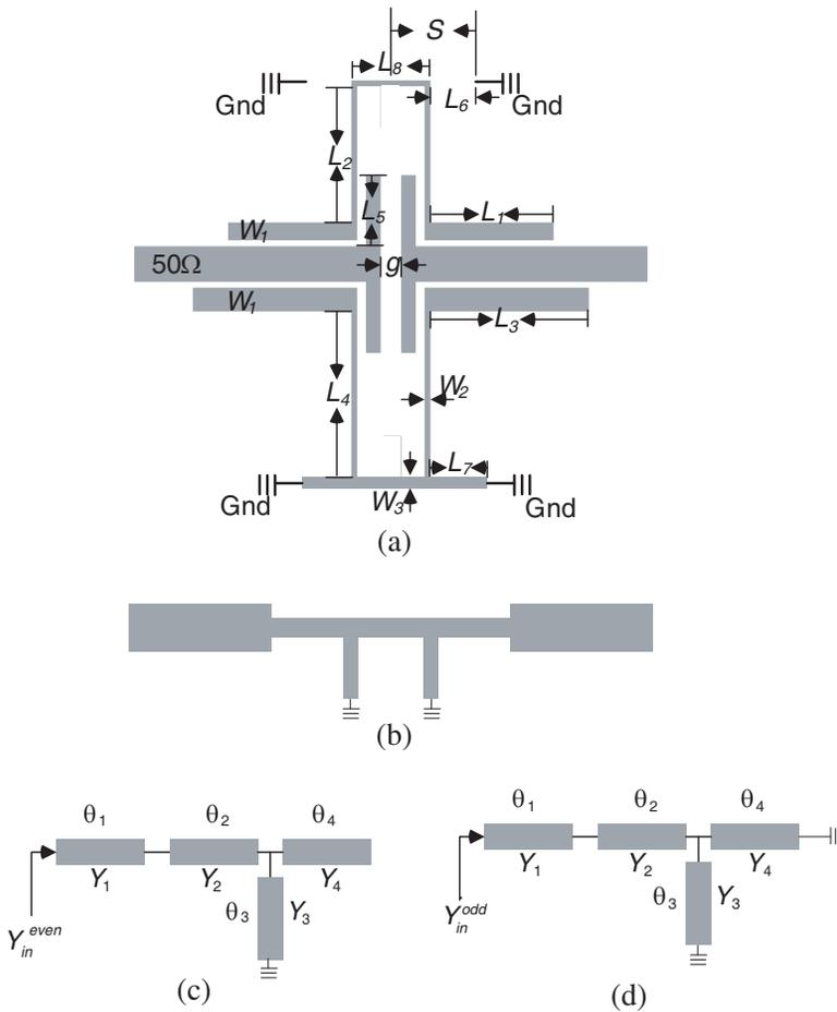
**Figure 1.** (a) Schematic of the quadruple-mode broadband BPF with source-load coupling. (b) Structure of the short-circuited stub-loaded SIR. (c) Even-mode equivalent circuit. (d) Odd-mode equivalent circuit.
