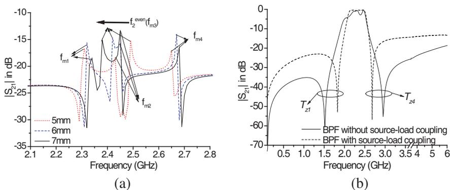
**Figure 2.** Simulated frequency-dependent transmission response of the presented BPF (a) Varying short-circuited stub-loaded  $S (L_6 + L_8/2)$ . (b) The quadruple-mode broadband BPF with and without source-load coupling.
