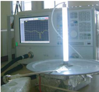
**Figure 1.** Experimental setup of plasma antenna for measuring return loss.
