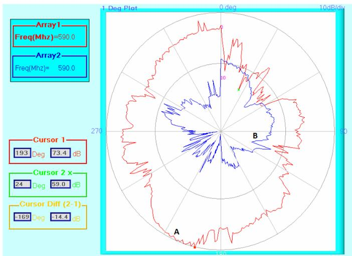
**Figure 10.** Radiation from the plasma antenna shows monopole patterns.
