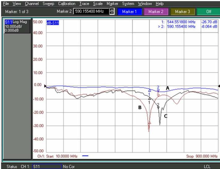
**Figure 6.** Response at 50 Hz AC voltage showing improved antenna characteristic but fluctuating resonant frequency.
