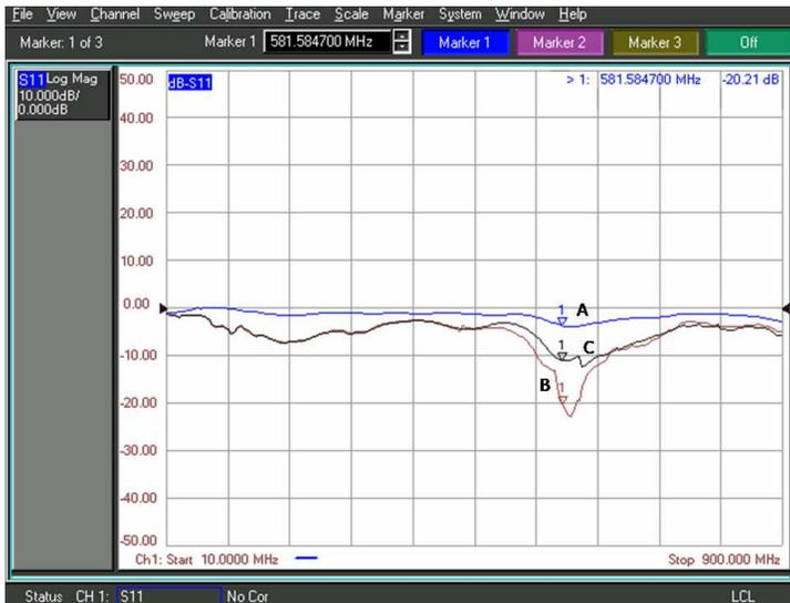
Figure 5. Response at 25 Hz AC voltage shows inefficient antenna characteristic.
