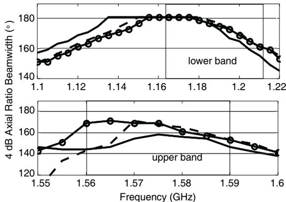
**Figure 2.** Simulated 4 dB axial ratio beamwidth as a function of the frequency for the dual-band antenna shown in Figure 1, for square substrate with  $D = 180$  mm (solid line), circular substrate with  $D = 180$  mm (solid line with circles) and circular substrate with  $D = 150$  mm (dashed line),  $\varphi = 0^\circ$  cut.
