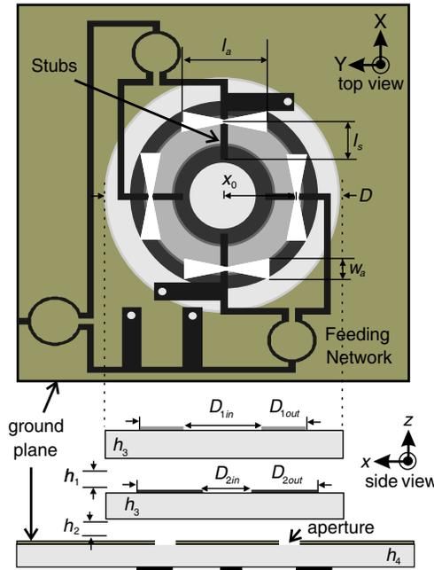
**Figure 1.** Geometry of the stacked annular-ring microstrip antenna.
