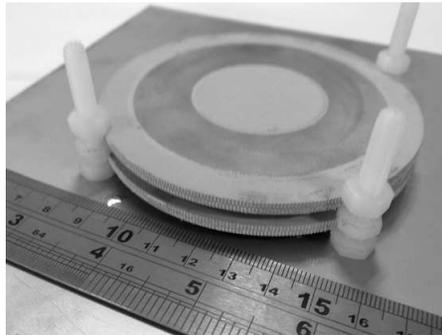
**Figure 3.** Fabricated antenna.
