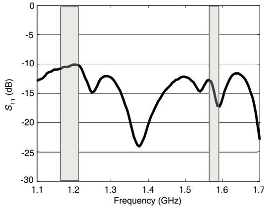
**Figure 4.** Measured input reflection coefficient for the fabricated dual-band circularly-polarized antenna.
