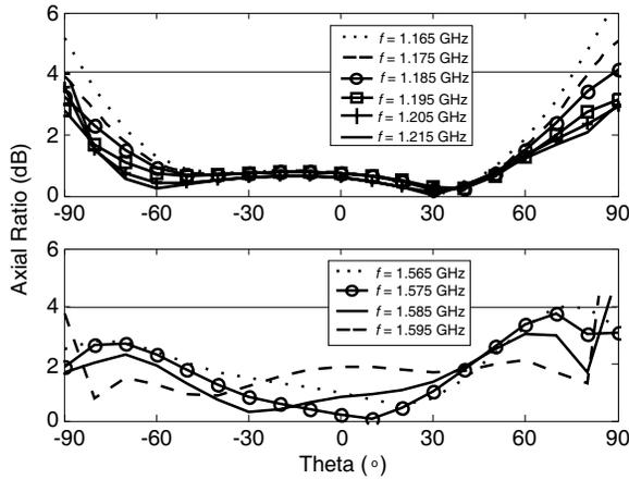
**Figure 6.** Simulated axial ratio as a function of angle  $\theta$ , for different frequency values,  $\varphi = 0^\circ$  cut.
