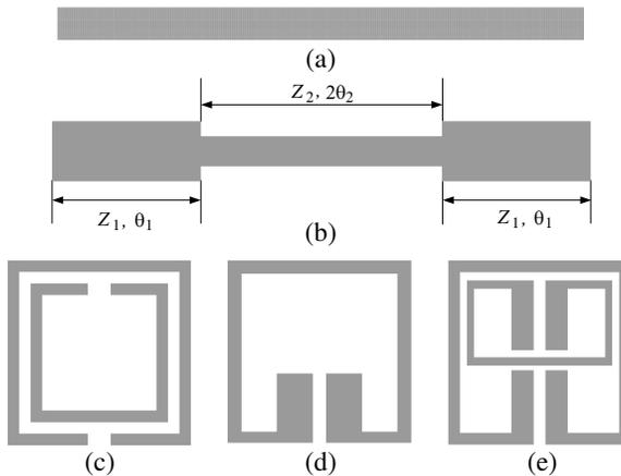
**Figure 1.** In each row of this figure represents the top view of a resonant magnetic particle. (a) UIR. (b) SIR. (c) SRRs. (d) SIR-SRR. (e) SIR-SRRs.
