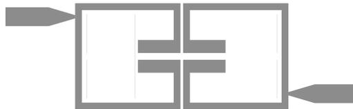
**Figure 2.** Geometry of the BPF with SIR-SRR.
