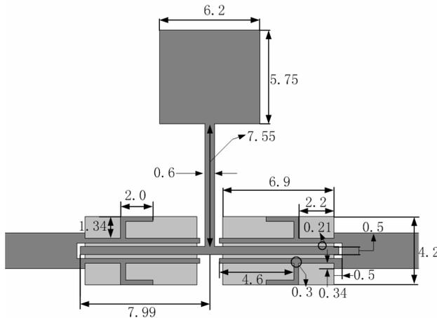
**Figure 1.** Configuration of the proposed UWB BPF (all in mm).
