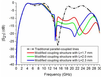
**Figure 3.** Frequency responses of the traditional parallel-coupled lines and the modified coupling structure.
