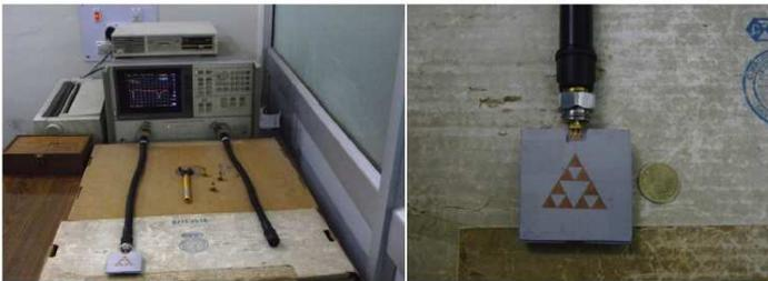
**Figure 9.** The fabricated antenna being tested on network analyzer.
