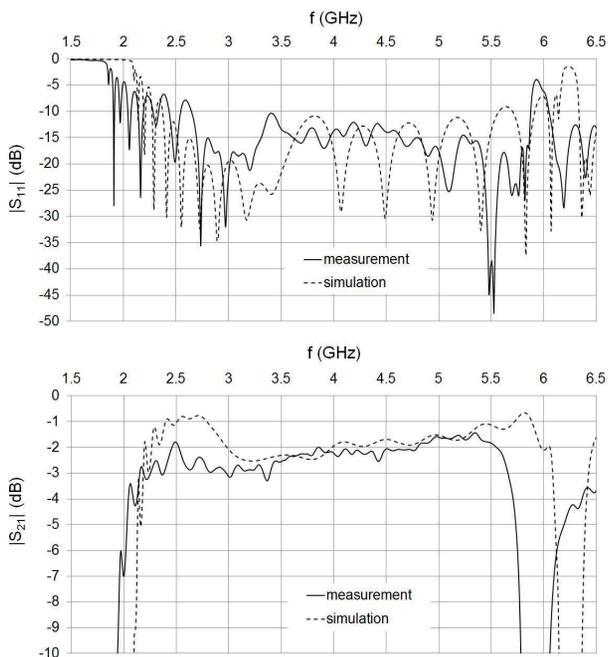
**Figure 6.** Return and insertion losses for the 10-cell prototype.
