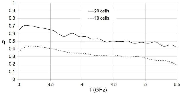
**Figure 7.** Efficiency versus frequency for the two prototypes.
