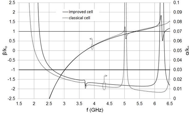
**Figure 4.** Propagation and attenuation factors normalized to  $k_0$ .
