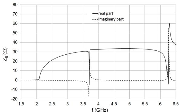
**Figure 5.** The Bloch impedance of the designed cell.
