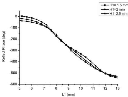
**Figure 2.** Phase responses of the proposed element for different  $H_1$  at the center frequency of 10 GHz ( $H_2 = 3$  mm,  $K = 0.66$ , and  $W = 0.3$  mm).
