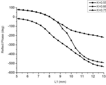
**Figure 4.** Phase responses of the proposed element for different  $K$  at the center frequency of 10 GHz ( $H_1 = 2$  mm,  $H_2 = 3$  mm, and  $W = 0.3$  mm).
