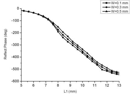
**Figure 5.** Phase responses of the proposed element for different  $W$  at the center frequency of 10 GHz ( $H_1 = 2$  mm,  $H_2 = 3$  mm, and  $K = 0.66$ ).
