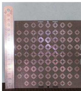
**Figure 7.** Photograph of the designed 77-element linear reflectarray.
