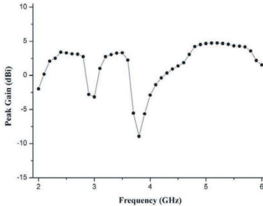
**Figure 6.** Gains of the antenna versus different frequencies.
