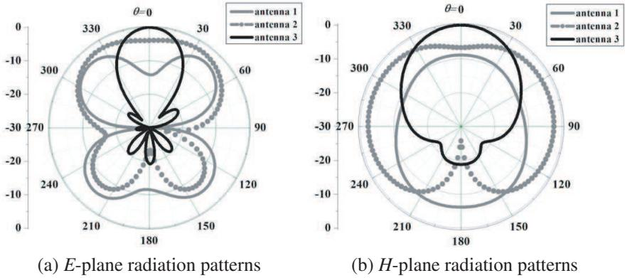
**Figure 2.** Simulated radiation patterns of different antenna structures.
