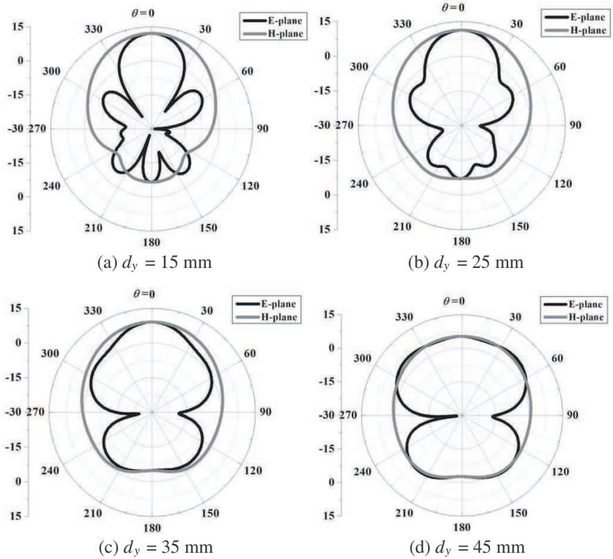
**Figure 3.** The simulated radiation patterns with different  $d_y$ .
