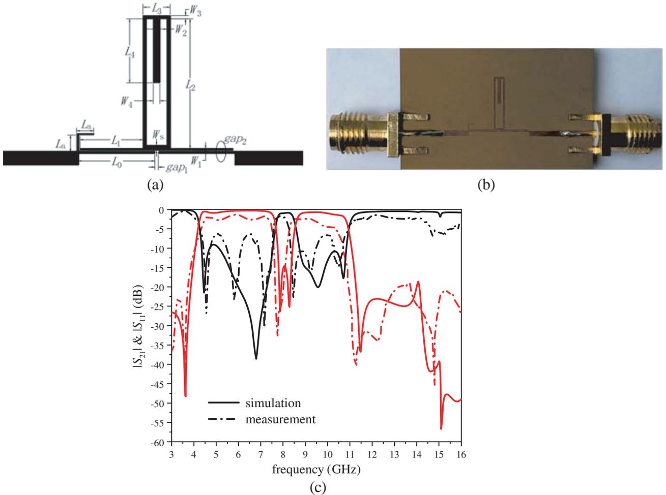
**Figure 4.** (a) Layout of the proposed filter. (b) Photo of the fabricated filter. (c) Simulated and measured results when  $W_1 = 0.1$  mm,  $W_2 = W_3 = 0.2$  mm,  $W_4 = W_s = 0.4$  mm,  $L_1 = 3.7$  mm,  $L_2 = 7.7$  mm,  $L_3 = 1.6$  mm,  $L_4 = 3.8$  mm,  $L_a = 1$  mm,  $gap_1 = 0.2$  mm, and  $gap_2 = 0.1$  mm.
