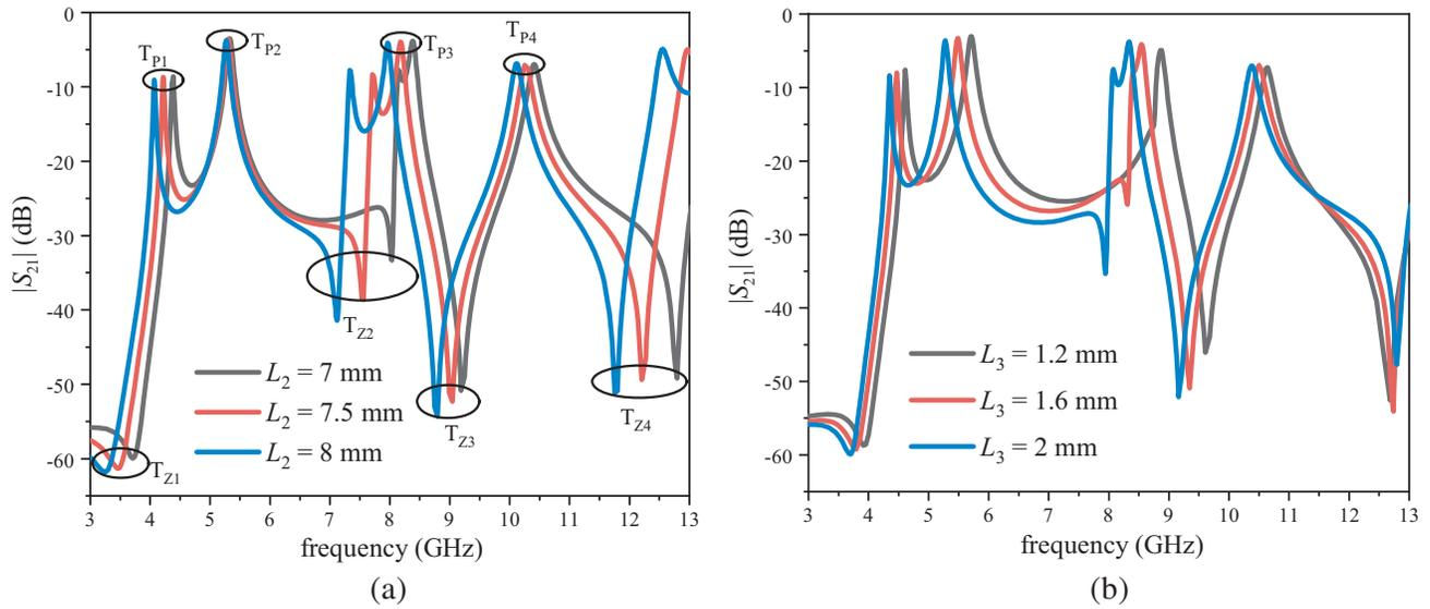
**Figure 2.** Simulated  $|S_{21}|$  of the proposed resonator under weak coupling. Different  $L_2$ ,  $L_3$ . (a) Different lengths  $L_2$  when  $L_1 = 4.5$  mm,  $L_3 = 1.9$  mm,  $L_4 = 3.3$  mm, and  $W = 0.2$  mm. (b) Different lengths  $L_3$  when  $L_1 = 4.5$  mm,  $L_2 = 7$  mm,  $L_4 = 3.3$  mm, and  $W = 0.2$  mm.
