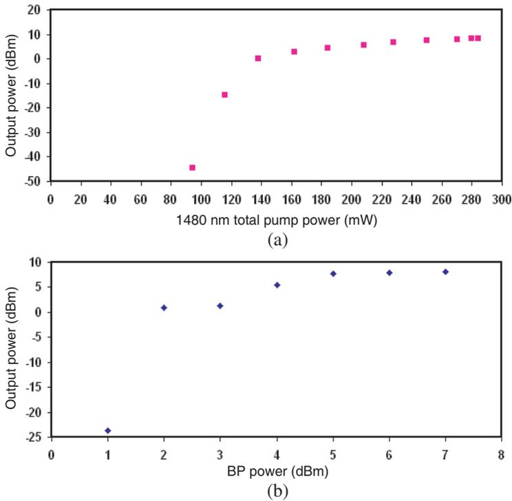
**Figure 4.** The peak power against the 1480 nm pump and BP powers. (a) 1480 nm pump, (b) BP.
