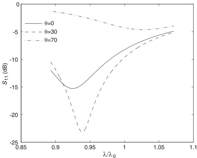
**Figure 5.** Simulated return loss of vee-antenna vs. frequency for different slope angles ( $\theta$ ).
