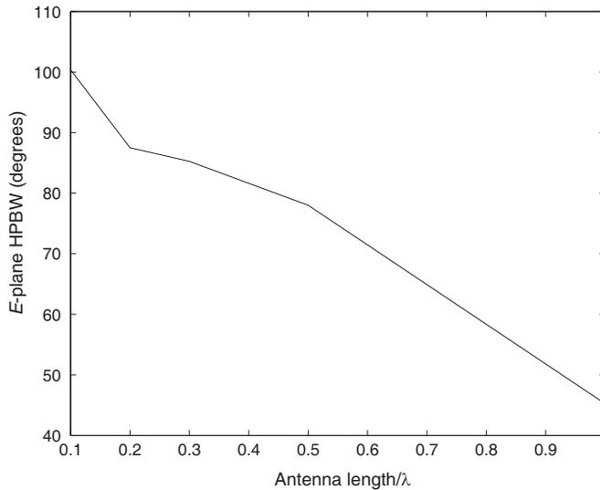
**Figure 2.** HPBW of a dipole antenna vs. its length (simulated with FEKO software).
