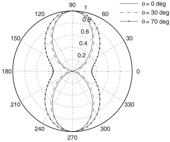
**Figure 7.** Radiation pattern of the resonant vee-antenna for different slope angles  $\theta$ .
