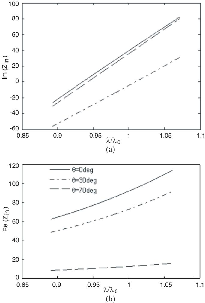
**Figure 6.** Imaginary (a) and real (b) part of the input impedance of resonant vee-antenna vs. frequency (simulated with FEKO software).
