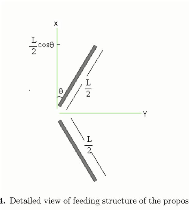
**Figure 4.** Detailed view of feeding structure of the proposed antenna.
