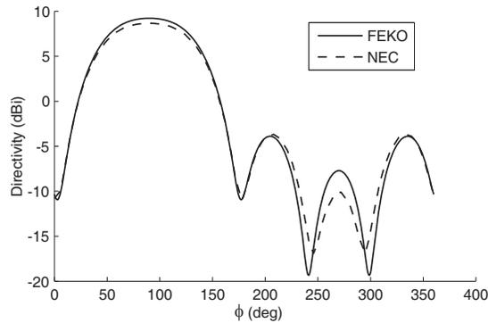
**Figure 11.** Simulated radiation pattern of the proposed antenna at  $f = f_0$ .
