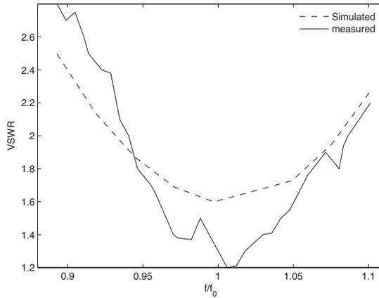
**Figure 10.** Simulated and measured VSWR of the fabricated antenna.
