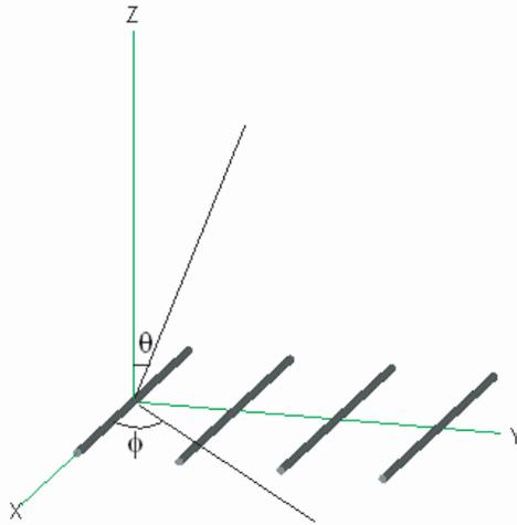
**Figure 1.** Yagi antenna as an array of dipoles.
