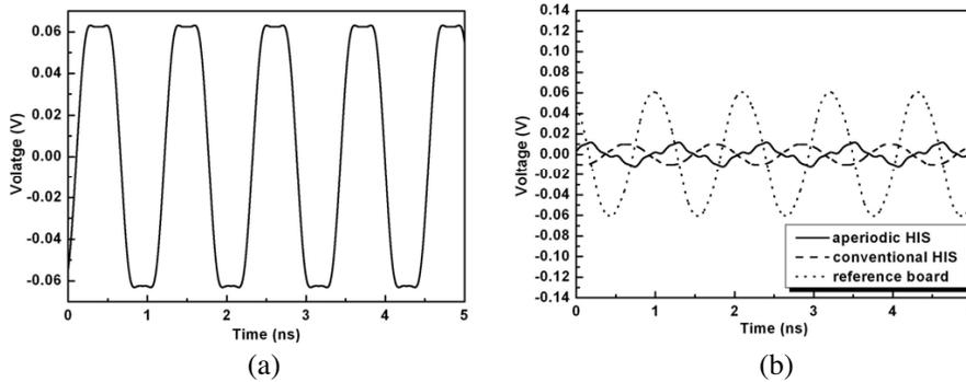
**Figure 6.** The SSN suppression performance in time domain. (a) Input current source. (b) Coupled noise at receiving port.
