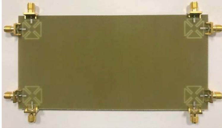
**Figure 12.** Fabricated smartphone antenna PCB.
