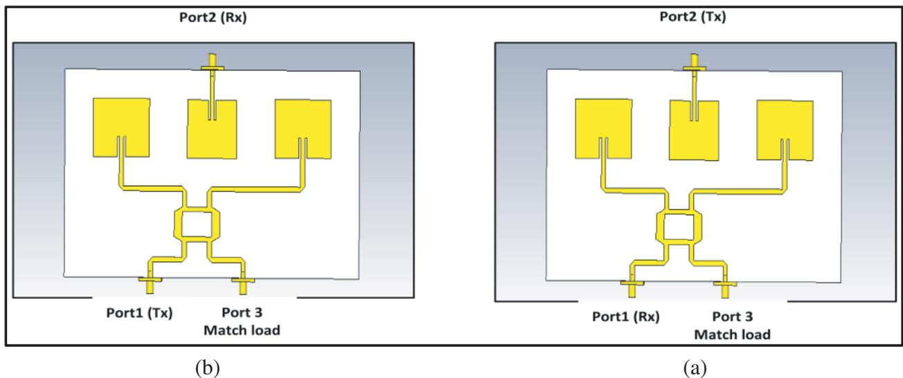
Figure 10. The two scenarios for transmitting the signal. (a) One transmit antenna and two receivers, (b) two transmit antennas and one receive.
