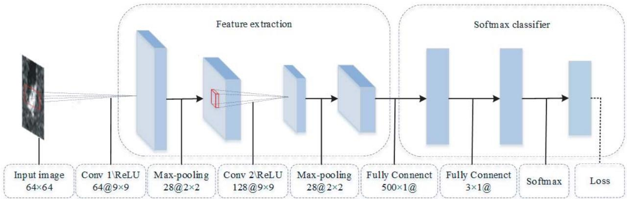
**Figure 1.** The diagram of the proposed network.
