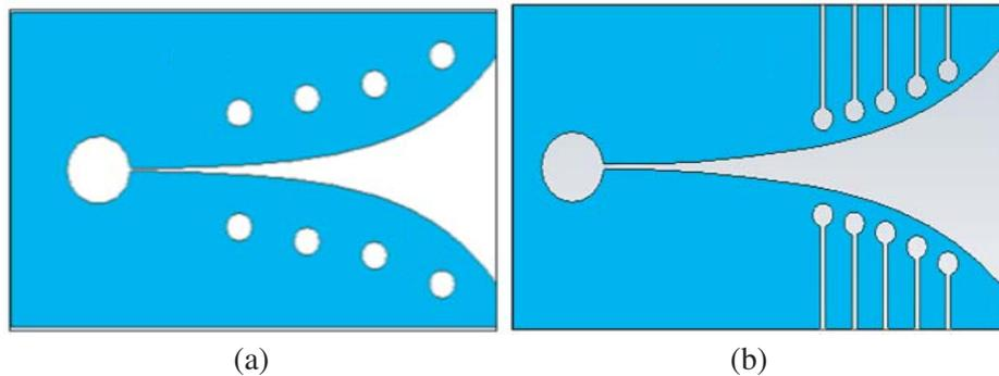
**Figure 6.** Vivaldi antenna by adding slot circles to the metal in (a) and Vivaldi antenna by adding slot circles and lines in (b).
