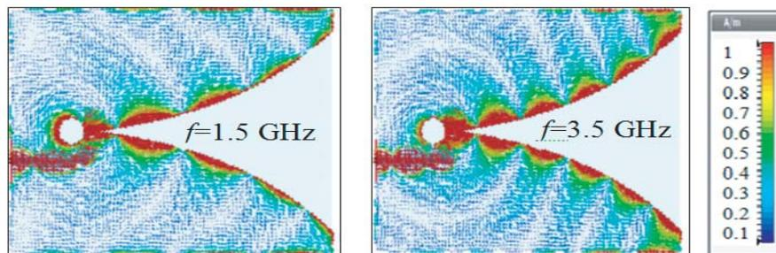
**Figure 5.** Current density for  $f = 1.5$  and  $f = 3.5$  GHz.
