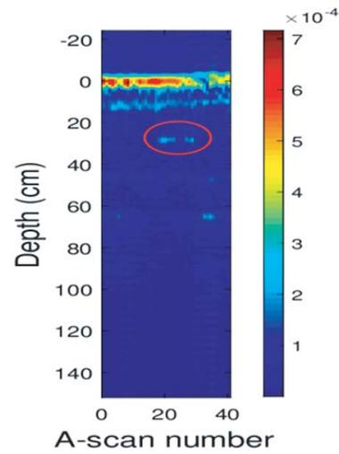
**Figure 16.** GPR detection using two plastic cylinders.
