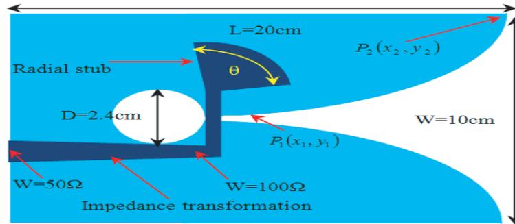
**Figure 1.** Vivaldi antenna (in front view) and its feeding line (in back view).
