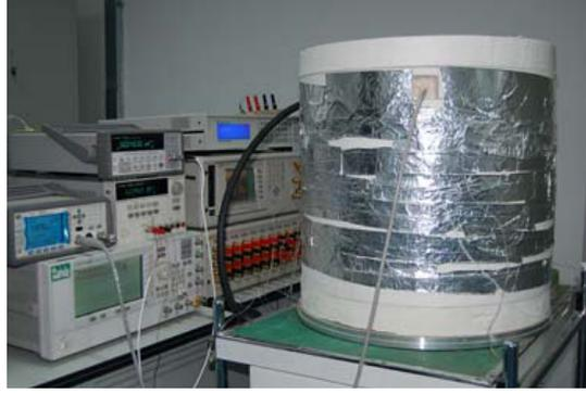
**Figure 11.** Measurement system of the calorimeter.
