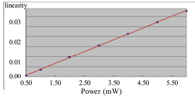
**Figure 9.** Fitted curve of the thermopile linearity.
