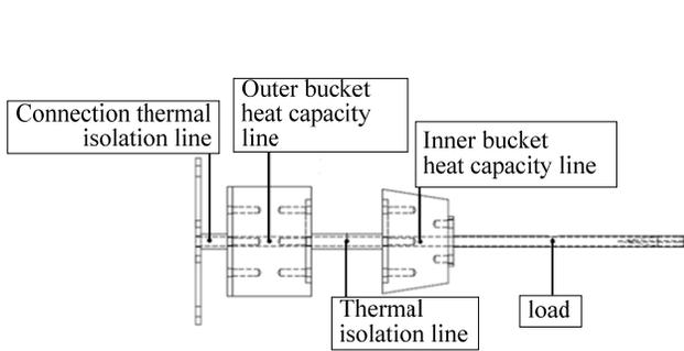
**Figure 6.** Thermal isolation line.
