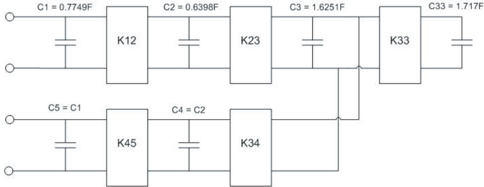
Figure 2. Inverter-coupled DBLPP configuration.
