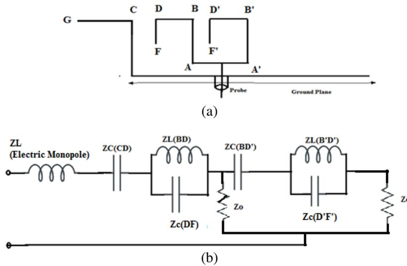
**Figure 4.** (a) Schematic of proposed magneto-electric monopole antenna. (b) Equivalent circuit of magneto-electric monopole antenna.
