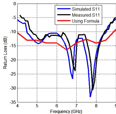
**Figure 6.** Measured, simulated and formula based return loss of proposed antenna.
