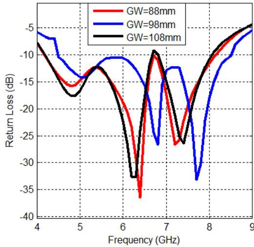
**Figure 14.** Simulated return loss of proposed antenna for different width of ground plane.
