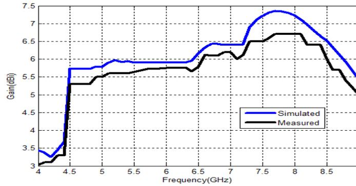
Figure 7. Measured and simulated gain of proposed antenna.
