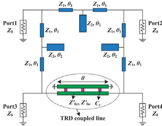
**Figure 2.** Configuration of the proposed rat-race coupler.
