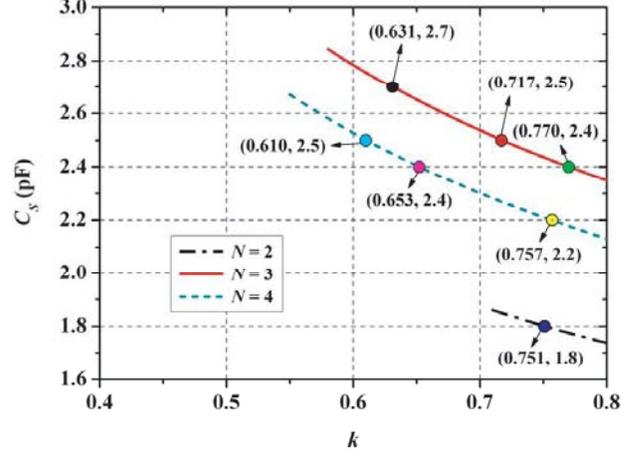
**Figure 4.** Required  $C_s$  of loaded capacitor as a function of  $k$ .
