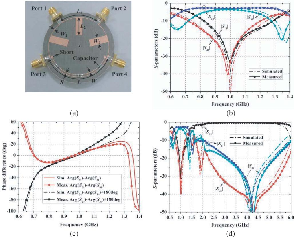
**Figure 7.** Photograph and  $S$ -parameters of the proposed 3-dB rat-race coupler. (a) Photograph. (b) Narrowband amplitude responses. (c) Narrowband phase responses. (d) Broadband amplitude responses.
