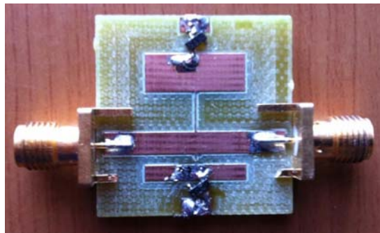
Figure 7. Fabricated DBBSF with tuning diode circuit.
