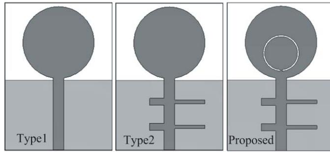
Figure 3. Step-wise evolution of the proposed antenna.
