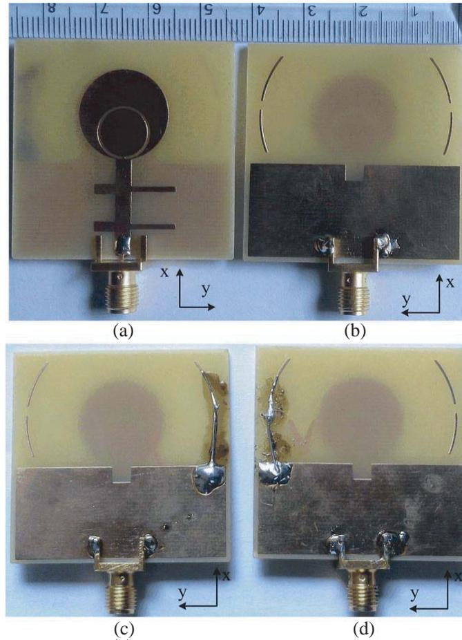
**Figure 7.** Prototype of the optimized antennas: (a) Top View, (b) bottom view at mode 0, (c) bottom view at mode 1, (d) bottom view at mode 2.
