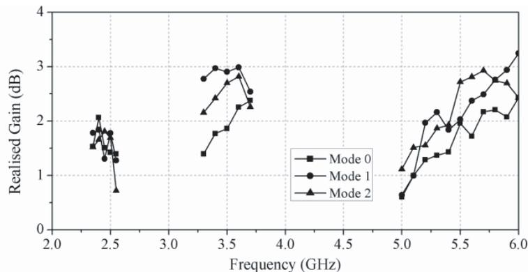
**Figure 10.** Measured realized gain of the proposed antenna.
