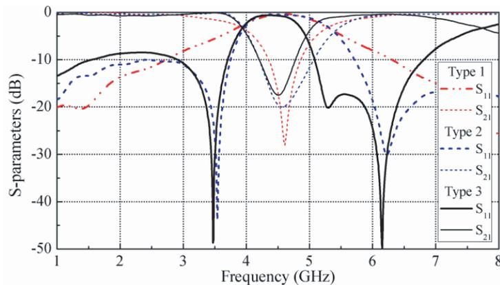
**Figure 2.** Simulated  $S$ -parameters of open-stub bandstop filters.
