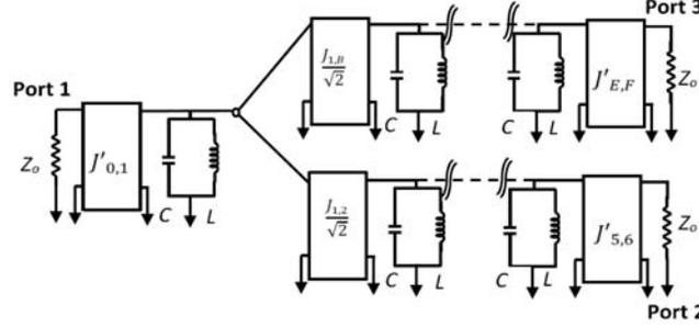
**Figure 3.** Equivalent circuit of a five-pole Chebyshev bandpass power splitter.
