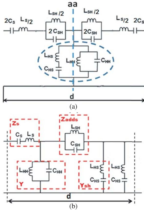
**Figure 1.** (a) The circuit model of conventional G NRI TL. (b) The circuit model of the proposed new asymmetric  $\pi$  G NRI TL.
