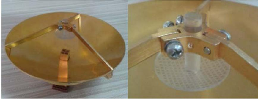
**Figure 7.** Photos of fabricated Cassegrain antenna.
