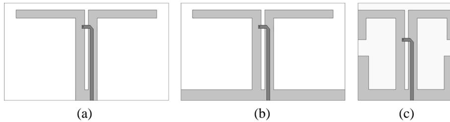
**Figure 2.** Design procedure for proposed antenna: (a) dipole only, (b) conventional QYA with dipole and reflector, and (c) proposed miniaturized QYA with folded parts in both ground reflector and driver dipole.
