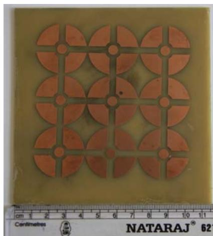
**Figure 2.** Prototype of proposed microstrip antenna.
