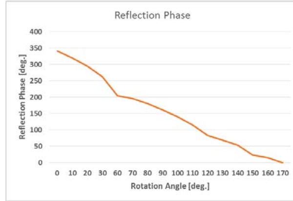
Figure 5. Reflection Phase of Pierrot cell against rotation about z -axis.
