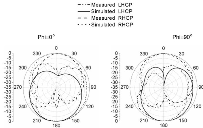
Figure 19. Simulated and measured radiation patterns at 3.1 GHz.
