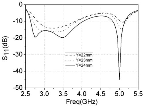
Figure 11. Simulated  $S_{11}$  with varying  $Y$ .
