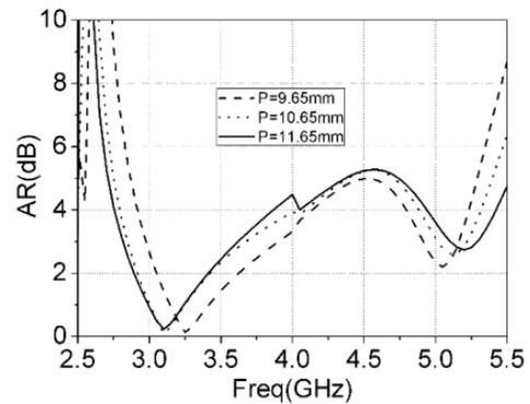
Figure 14. Simulated AR with varying  $P$ .
