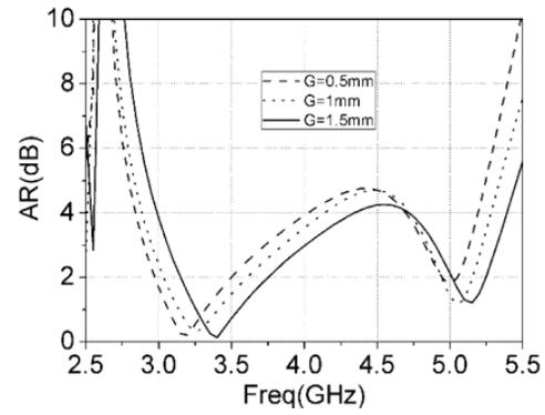
Figure 8. Simulated AR with varying  $G$ .
