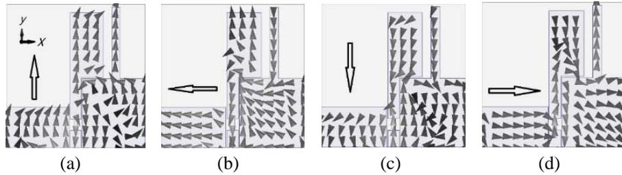
**Figure 3.** Simulated surface vector current distribution of proposed antenna at 3.3 GHz for four phases, (a)  $0^\circ$ , (b)  $90^\circ$ , (c)  $180^\circ$ , (d)  $270^\circ$ .
