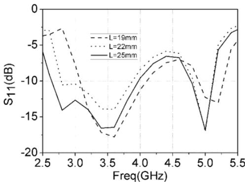
Figure 15. Simulated  $S_{11}$  with varying  $L$ .
