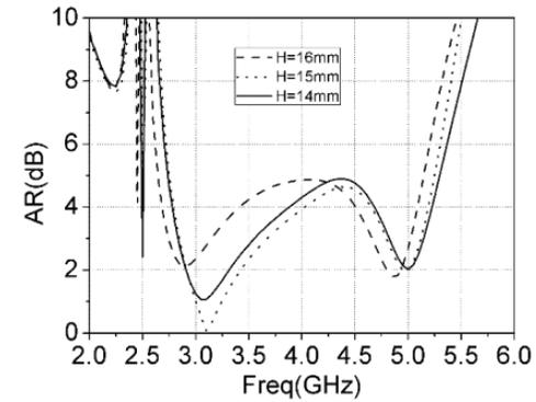
Figure 10. Simulated AR with varying  $H$ .
