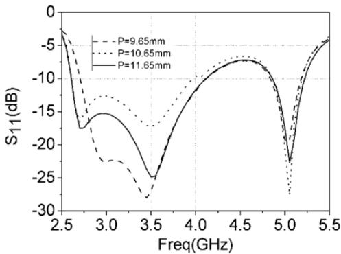
Figure 13. Simulated  $S_{11}$  with varying  $P$ .
