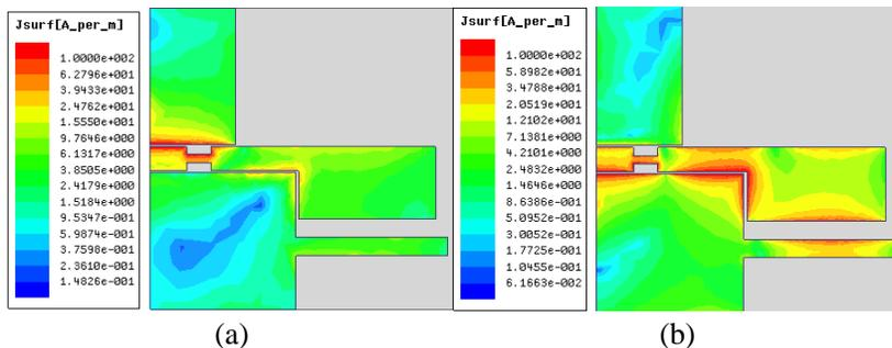
Figure 2. Current distribution at (a) 3.3 GHz and (b) 5.1 GHz.
