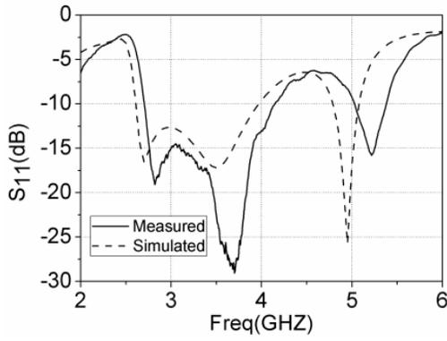
Figure 17. Simulated and measured  $S_{11}$ .
