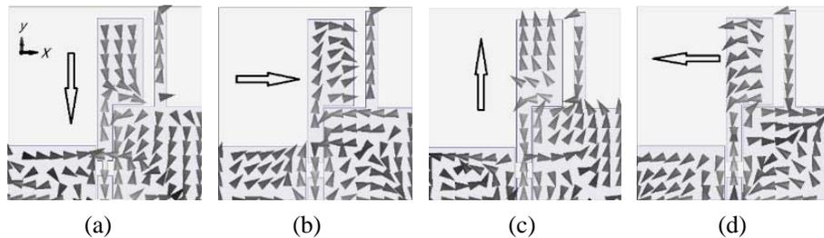
**Figure 4.** Simulated surface vector current distribution of proposed antenna at 5.1 GHz for four phases, (a)  $0^\circ$ , (b)  $90^\circ$ , (c)  $180^\circ$ , (d)  $270^\circ$ .
