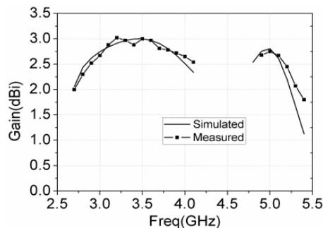
Figure 21. Simulated and measured gain in  $+z$  direction.
