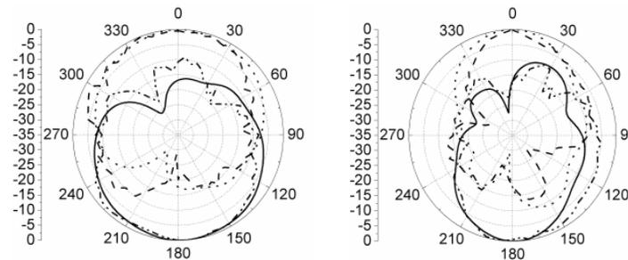
Figure 20. Simulated and measured radiation patterns at 5.1 GHz.
