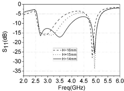
Figure 9. Simulated  $S_{11}$  with varying  $H$ .
