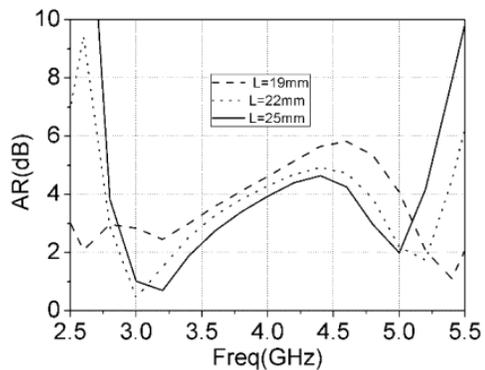
Figure 16. Simulated AR with varying  $L$ .
