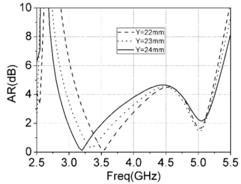
Figure 12. Simulated AR with varying  $Y$ .
