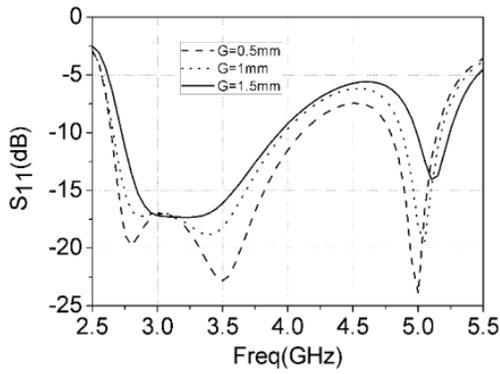
Figure 7. Simulated  $S_{11}$  with varying  $G$ .
