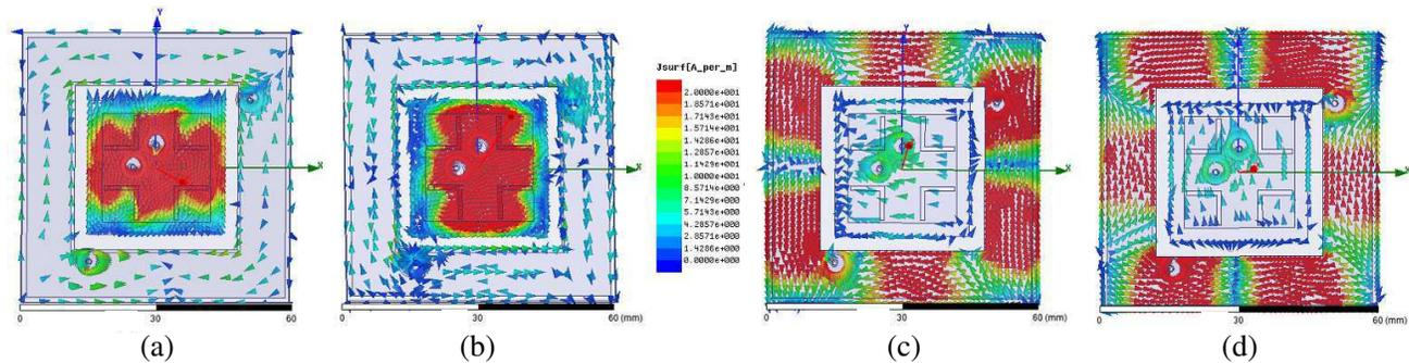
**Figure 8.** Current distribution of antenna at 2.45 GHz for each port: (a) Port 1, (b) Port 2, (c) Port 3, and (d) Port 4.
