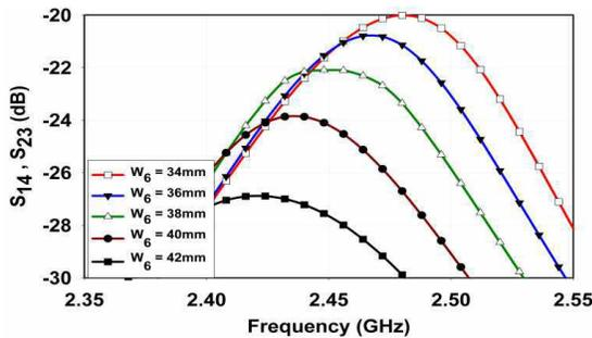
Figure 4. Parametric study of  $S_{14}$  and  $S_{23}$  with DGS length.
