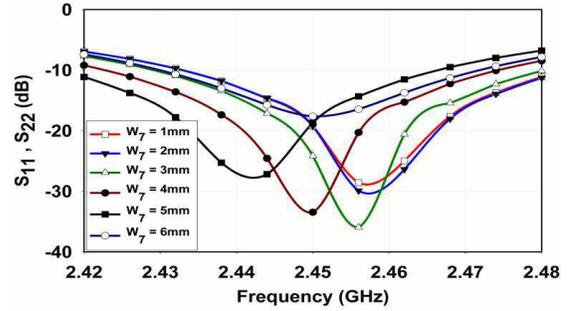
**Figure 7.** Parametric study of  $S_{11}$  and  $S_{22}$  with DGS width.
