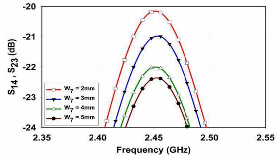
Figure 5. Parametric study of  $S_{14}$  and  $S_{23}$  with DGS width.
