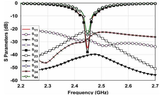
Figure 9. Simulated  $S$  parameters without DGS.
