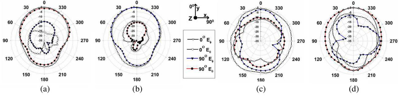
**Figure 13.** Measured radiation pattern in  $0^\circ$  plane and  $90^\circ$  plane for each ports: (a)  $P_1$ , (b)  $P_2$ , (c)  $P_3$ , and (d)  $P_4$ .
