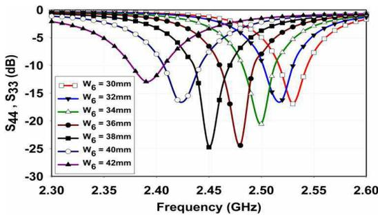
**Figure 6.** Parametric study of  $S_{33}$  and  $S_{44}$  with DGS length.
