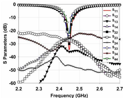
Figure 12. Measured  $S$  parameters of four-port antenna.
