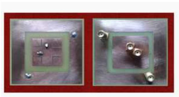
Figure 11. Prototype of antenna (top and bottom view).
