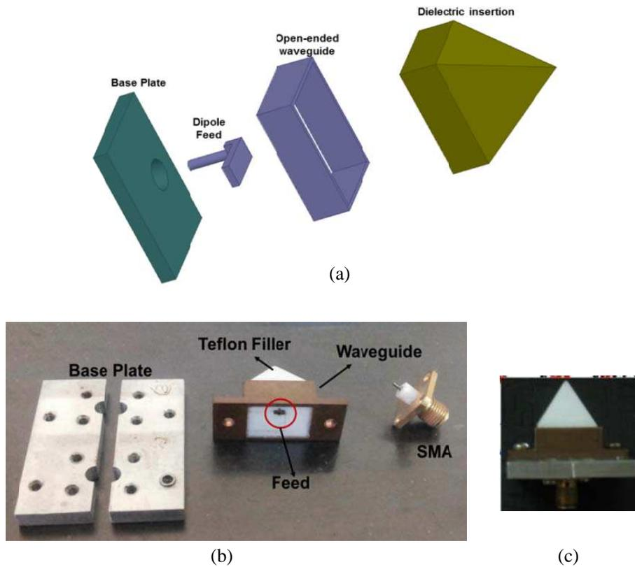
**Figure 5.** Assembly scheme of the MLA structure, (a) assembly scheme, (b) photograph of different parts of MLA assembly, (c) assembled view of MLA.
