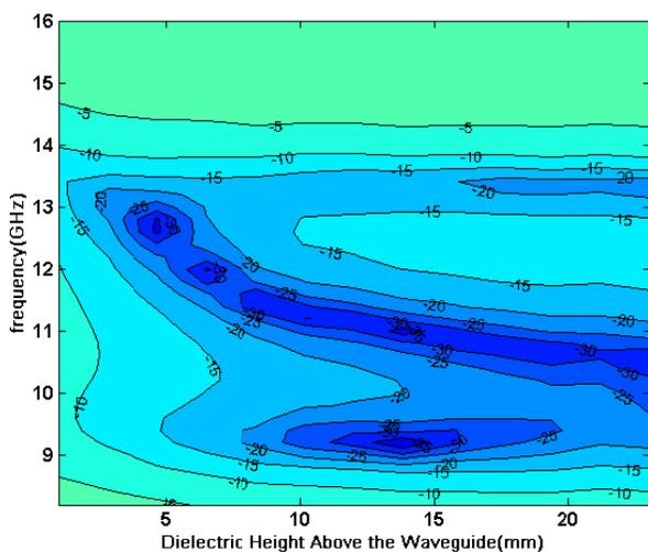
**Figure 2.** Variation of reflection coefficient w.r.t. dielectric height over the frequency band.
