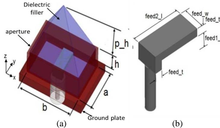
**Figure 1.** HFSS models of (a) proposed MLA and (b) VED feed structures.
