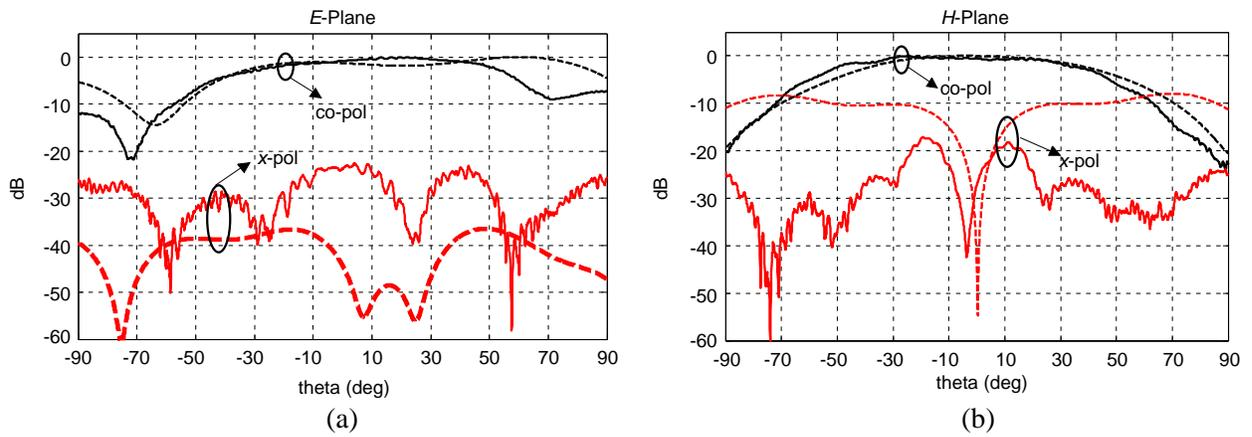
**Figure 8.** Radiation pattern plots of MLA (Measured trace (solid) and simulated trace (dash)), (a) in *E*-plane, (b) in *H*-plane.
