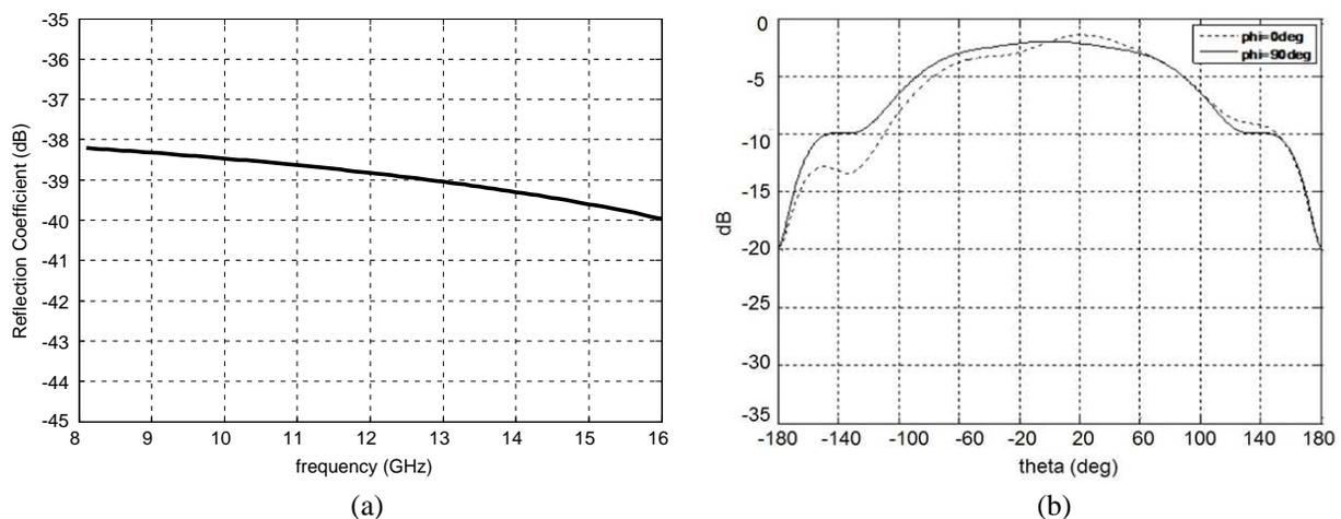
**Figure 6.** (a) Simulated return loss plot of VED and (b) simulated radiation pattern plots of VED feed.
