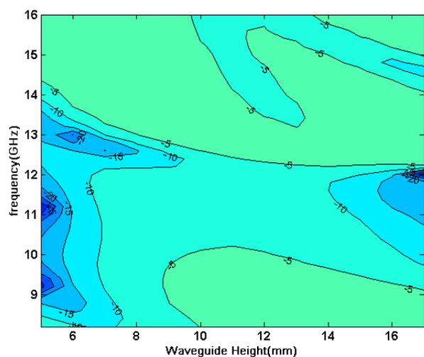
**Figure 3.** Variation of reflection coefficient w.r.t. waveguide height over the frequency band.
