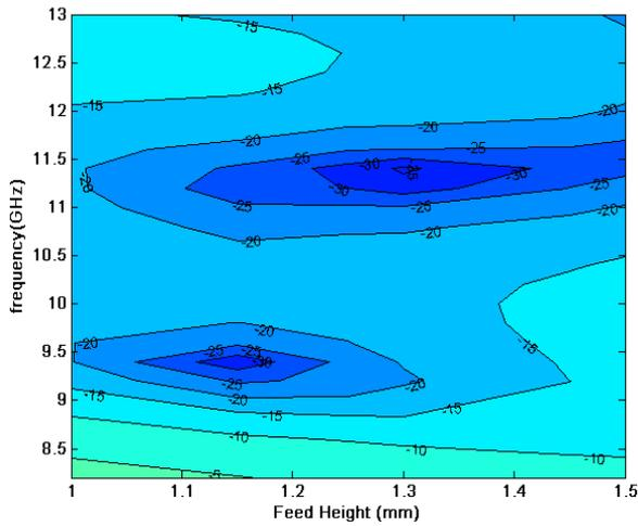
**Figure 4.** Variation of reflection coefficient w.r.t. feed height over the frequency band.
