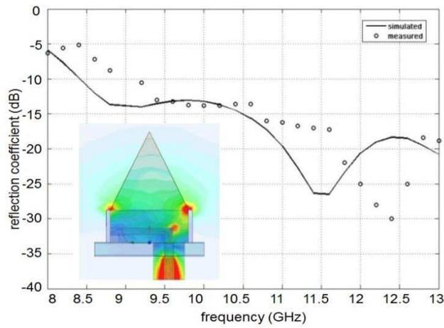
**Figure 7.** Measured and simulated reflection coefficient plots of antenna. (Inset shows the current distribution on the antenna structure).
