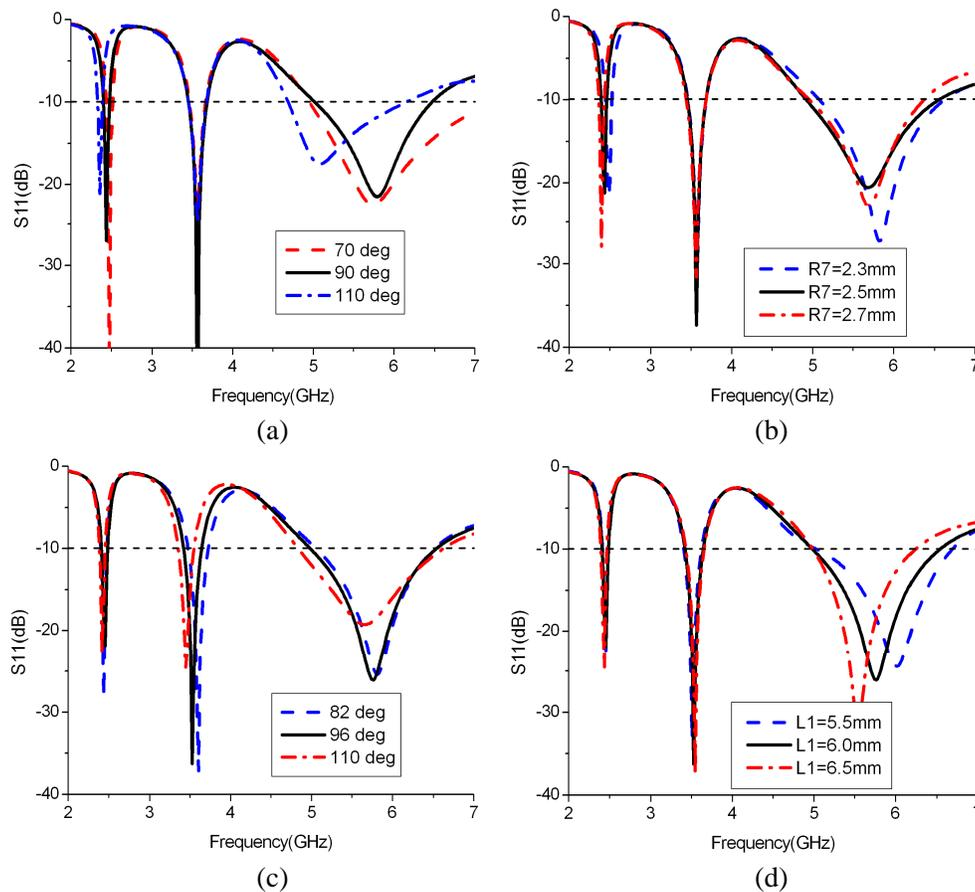
**Figure 3.** Simulated reflection coefficient of the proposed antenna. (a) When the central angle of  $\varphi$  changes. (b) When the length of  $R_7$  changes. (c) When the central angle of  $\beta$  changes. (d) When the length of  $L_1$  changes.
