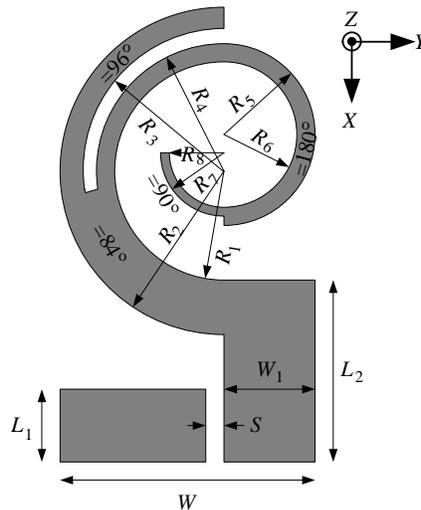
**Figure 1.** Geometry of the proposed ACS-fed monopole antenna.
