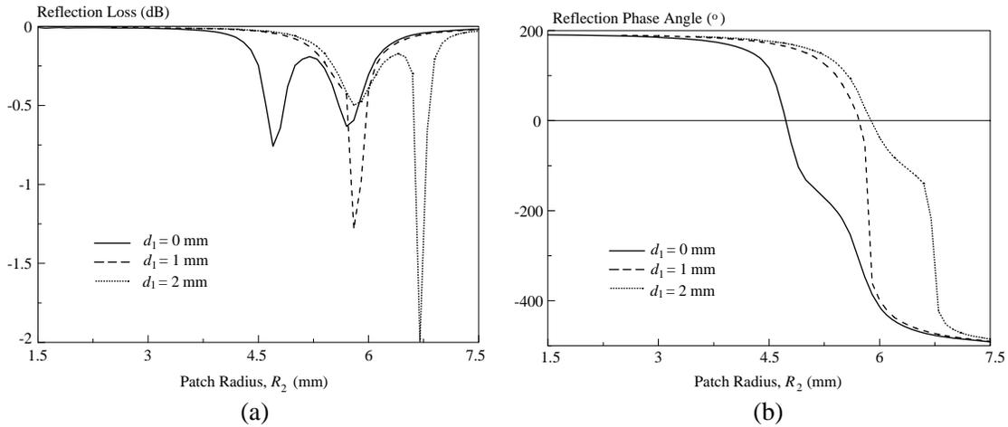
**Figure 8.** Effects of the radius difference  $d_1$  (where  $R_2 > R_1$ ) on the (a) reflection loss; (b) reflection phase angle of the proposed double-layered reflectarray unit element.
