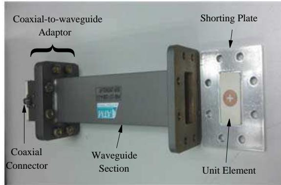
**Figure 3.** Experimental setup of the waveguide model.
