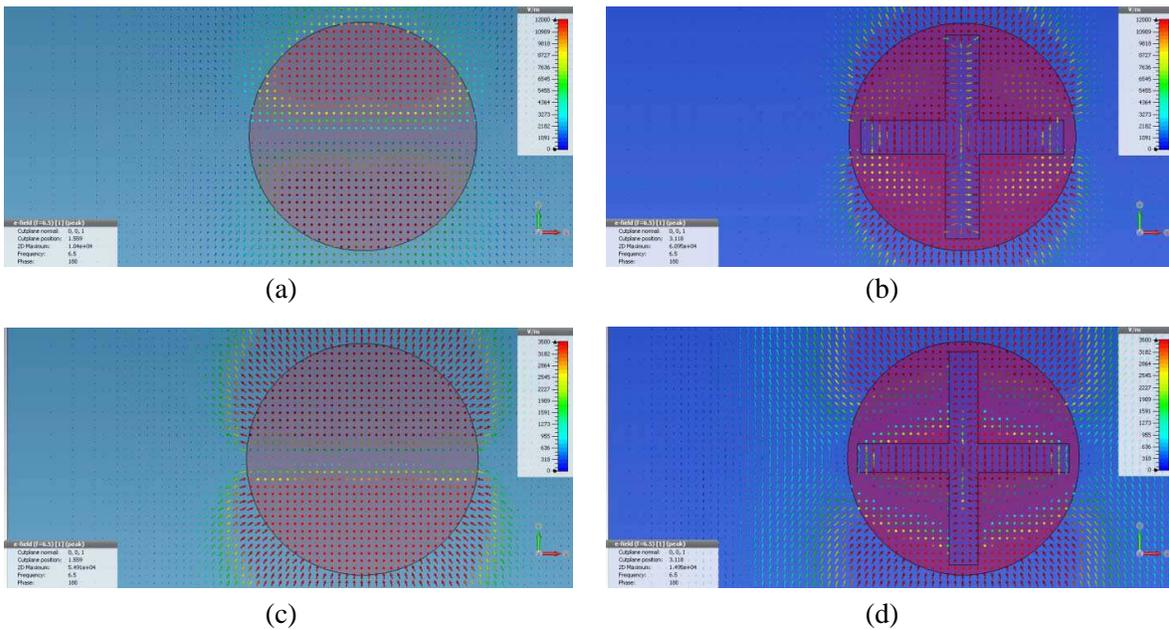
**Figure 5.** Electric field distributions between (a) middle patch and ground at  $R_1 = R_2 = 4.7$  mm, (b) top and middle patch at  $R_1 = R_2 = 4.7$  mm, (c) middle patch and ground at  $R_1 = R_2 = 5.7$  mm, (d) top and middle patch at  $R_1 = R_2 = 5.7$  mm.
