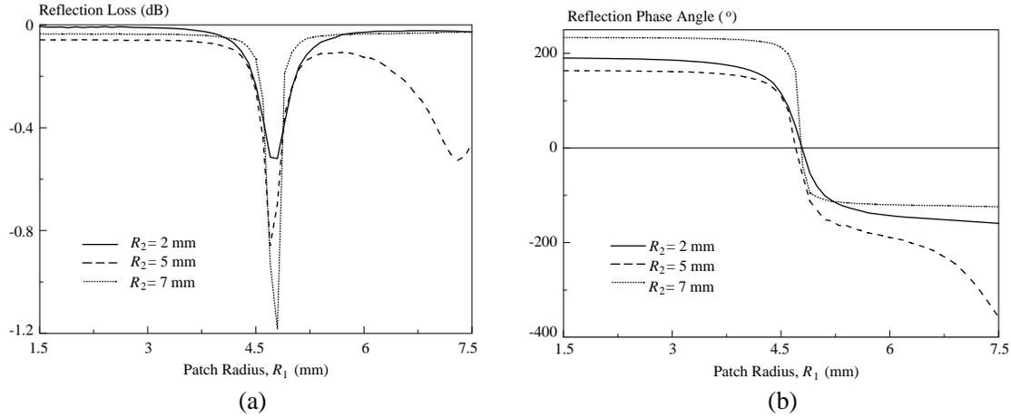
**Figure 7.** Effects of the middle circular patch radius ( $R_2$ ) on the (a) reflection loss; (b) reflection phase angle of the proposed double-layered reflectarray unit element.
