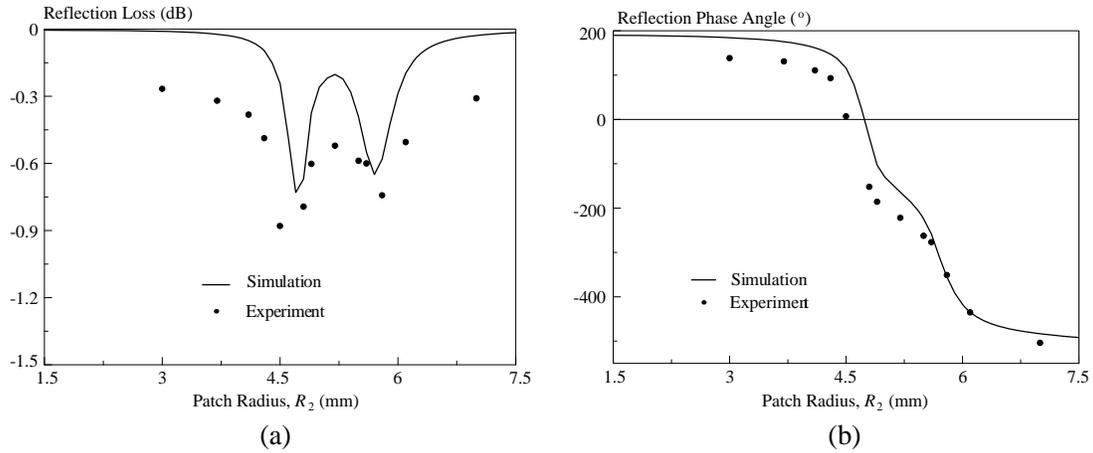
**Figure 4.** Measured and simulated (a) reflection losses, (b) reflection phase angles of the proposed double-layered reflectarray unit element.
