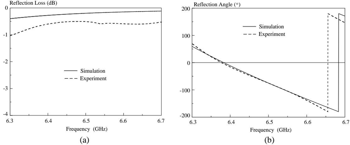
**Figure 6.** Measured and simulated (a) reflection coefficients, (b) angles of reflection against frequency for  $R_1 = R_2 = 6.1$  mm of the proposed double-layered reflectarray unit element.
