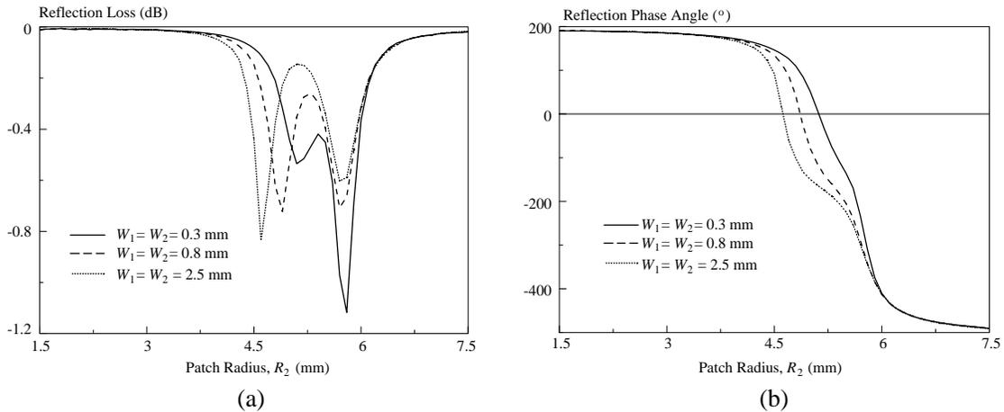
**Figure 9.** Effects of the slot widths ( $W_1, W_2$ ) on the (a) reflection loss; (b) reflection phase angle of the proposed double-layered reflectarray unit element.
