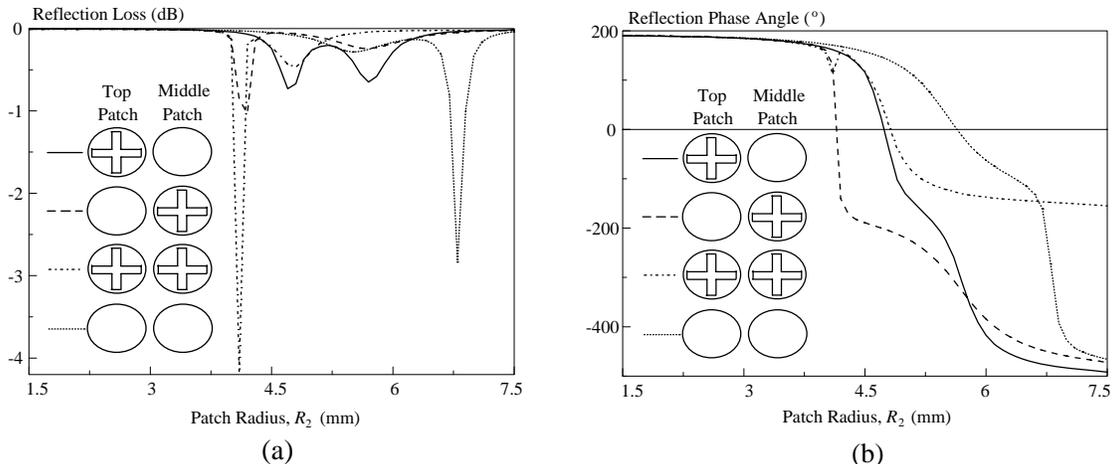
**Figure 12.** Different combinations of top and middle circular patches on the (a) reflection loss; (b) reflection phase angle.
