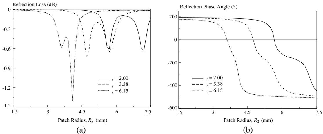
**Figure 11.** Effects of the substrate dielectric constant  $\epsilon_r$  on the (a) reflection loss; (b) reflection phase angle of the proposed double-layered reflectarray unit element.
