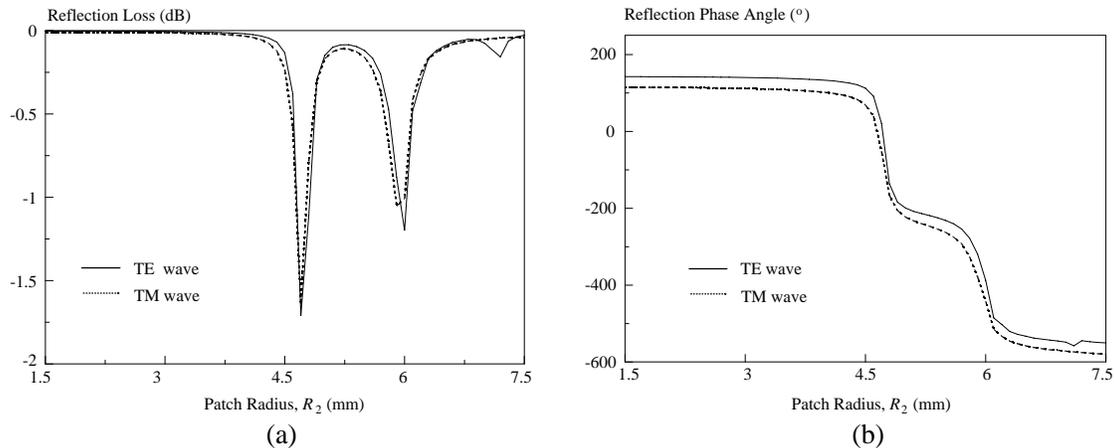
**Figure 13.** (a) Reflection losses and (b) reflection phase angles for the TE- and TM-polarized incoming waves.
