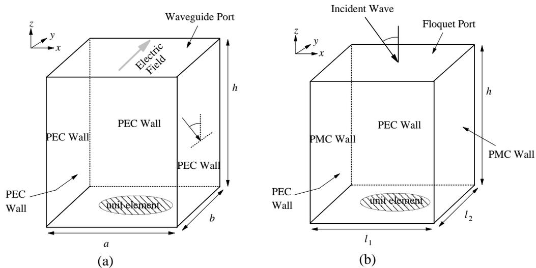
**Figure 2.** (a) Waveguide model. (b) Floquet model.
