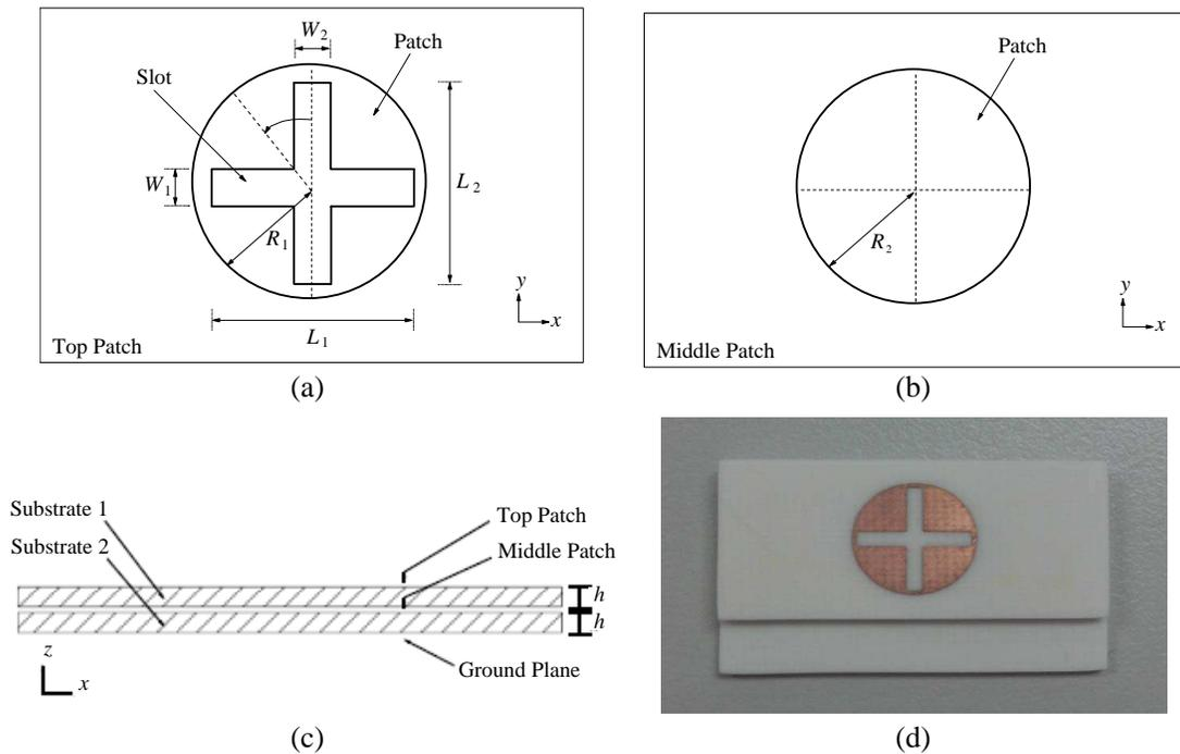
**Figure 1.** Double-layered microstrip reflectarray unit element. (a) Top patch. (b) Middle patch. (c) Side view. (d) Photograph of the fabricated prototype.
