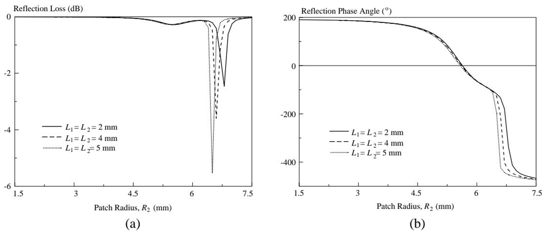
**Figure 10.** Effects of the slot lengths ( $L_1, L_2$ ) on the (a) reflection loss; (b) reflection phase angle of the proposed double-layered reflectarray unit element.
