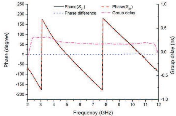
**Figure 11.** Measured phase difference and group delay.
