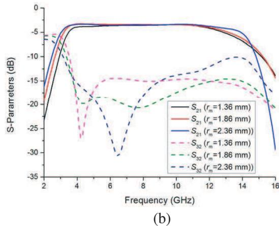
**Figure 5.** The influence of  $r_m$  on frequency response. (a) The influence on return losses at input and output ports. (b) The influence on insertion loss and isolation.
