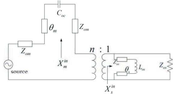
**Figure 2.** Equivalent circuit of the microstrip-to-slotline transition.
