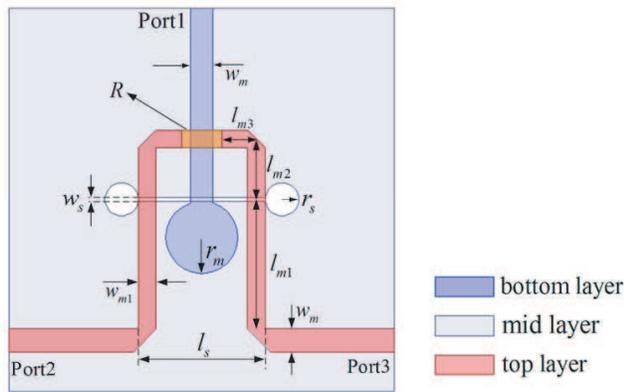
**Figure 3.** Configuration of the UWB multilayer power divider.
