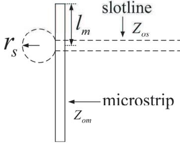
**Figure 1.** Model of microstrip-to-slotline transition.
