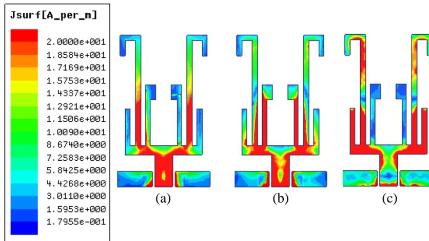
Figure 3. Simulated surface current distribution of the proposed antenna at (a) 2.5 GHz, (b) 3.5 GHz, (c) 5.5 GHz.
