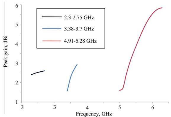
**Figure 8.** Peak gain of the proposed antenna.
