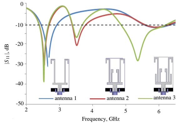
Figure 2. Simulated reflection coefficient of involved antennas.
