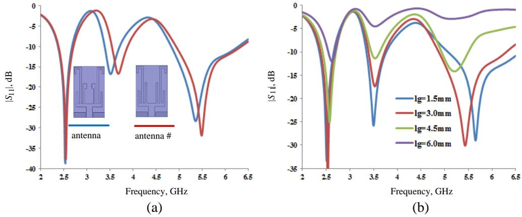
**Figure 5.** (a) Simulated reflection coefficients of the proposed antenna and antenna #. (b) Simulated reflection coefficients of the proposed antenna with varied  $l_g$ .
