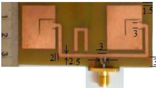
**Figure 12.** Two element array with DGS and resonator (dimensions are in mm).
