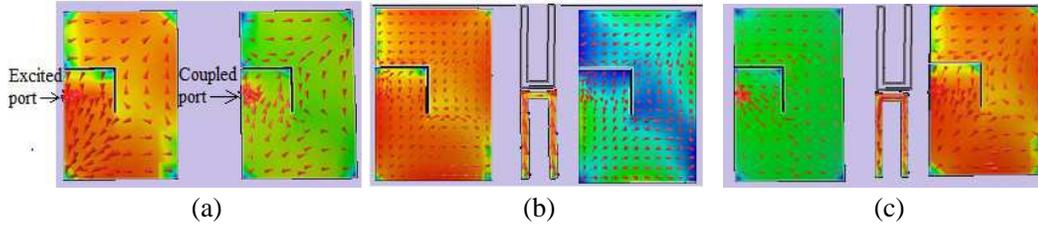
**Figure 5.** Simulated current distributions at 2.45 GHz, (a) antenna-1 is excited without resonator and DGS, (b) antenna-1 is excited with resonator and DGS, and (c) antenna-2 is excited with resonator and DGS.
