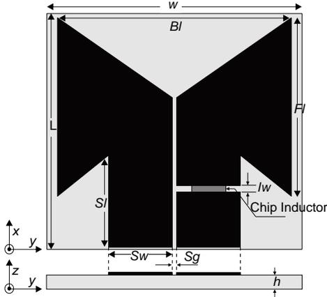
**Figure 1.** Geometry of proposed antenna,  $Bl = 11 \text{ mm}$ ,  $Fl = 8.4 \text{ mm}$ ,  $Sl = 4 \text{ mm}$ ,  $Sw = 3 \text{ mm}$ ,  $Sg = 0.2 \text{ mm}$ ,  $Iw = 0.3 \text{ mm}$ ,  $h = 1.6 \text{ mm}$ ,  $L = 11.1 \text{ mm}$ ,  $W = 12 \text{ mm}$ .
