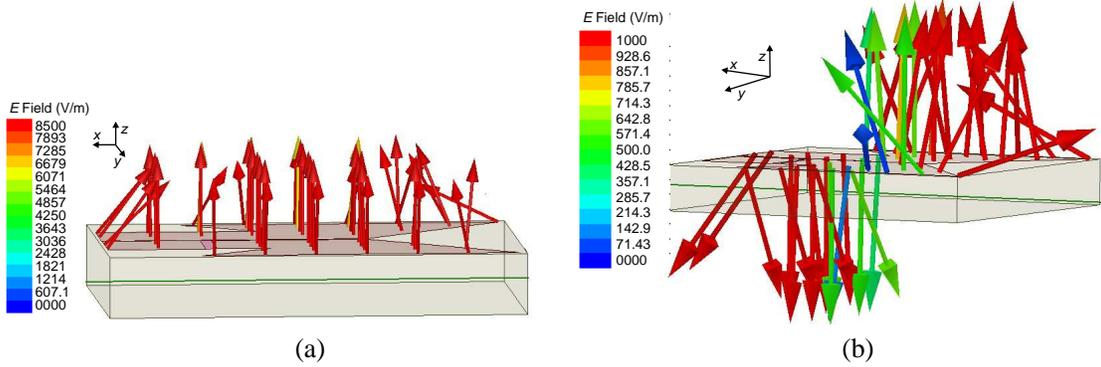
**Figure 5.** Electric field distribution, (a) at  $n = 0$  mode, (b) at  $n = +1$  mode,  $Bl = 11$  mm,  $Fl = 8.4$  mm,  $Sl = 4$  mm,  $Sw = 3$  mm,  $Sg = 0.2$  mm,  $Iw = 0.3$  mm,  $h = 1.6$  mm,  $L = 11.1$  mm,  $W = 12$  mm.
