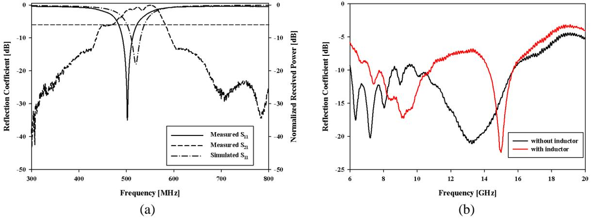
**Figure 4.** (a) Transmission and reflection characteristics of antenna. (b) Reflection coefficient of bowtie antenna with and without inductor,  $Bl = 11$  mm,  $Fl = 8.4$  mm,  $Sl = 4$  mm,  $Sw = 3$  mm,  $Sg = 0.2$  mm,  $Iw = 0.3$  mm,  $h = 1.6$  mm,  $L = 11.1$  mm,  $W = 12$  mm.
