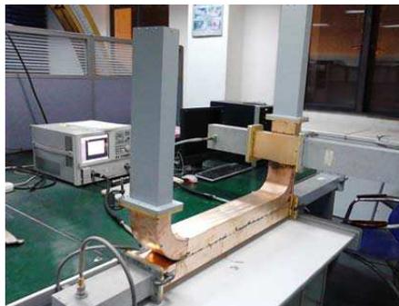
**Figure 8.** The measurement photo of the coupling degree of TSCDC.
