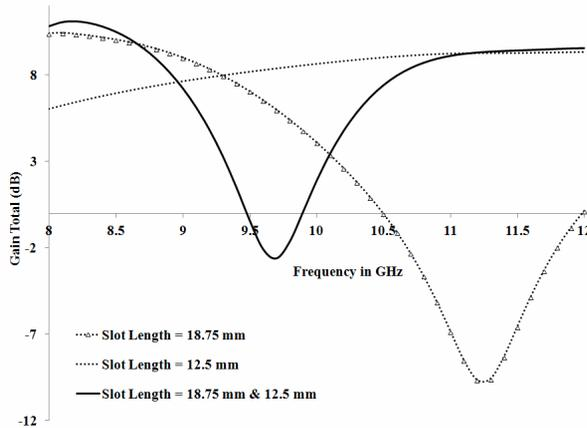
**Figure 7.** Plot of gain versus frequency at Theta = 0 and Phi = 0 direction for three slot array antennas, one with non-uniform length (18.75 mm & 12.5 mm) and two with uniform lengths (18.75 mm & 12.5 mm respectively).
