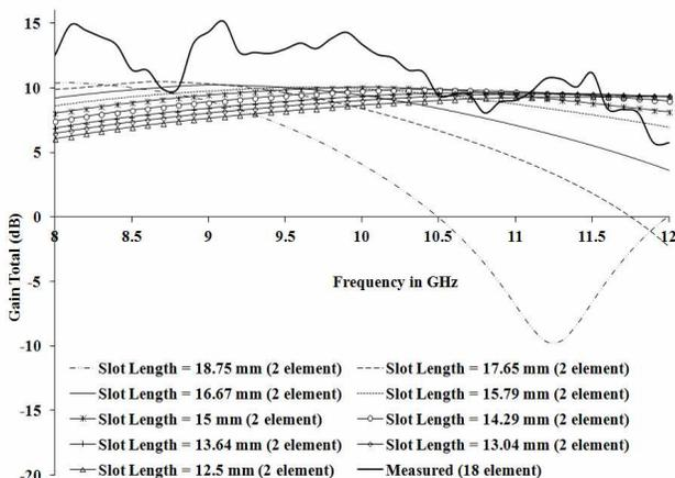
Figure 9. Plot of gain as a function of frequency at  $\Theta = 0$  and  $\Phi = 0$  direction for the 18-element slot array and nine other two-element slot arrays corresponding to resonance frequencies 8, 8.5, 9, 9.5, 10, 10.5, 11, 11.5 and 12 GHz respectively.
