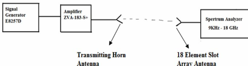
Figure 8. Block diagram of the experimental setup for measurement.
