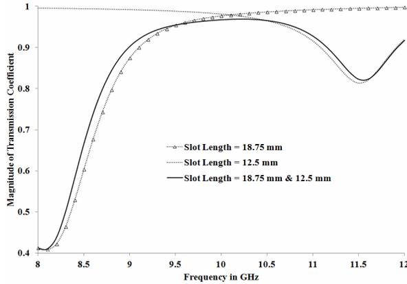
**Figure 6.** Variation of magnitude of transmission coefficients with frequency for three slot array antennas, one with non-uniform length (18.75 mm & 12.5 mm) and two with uniform lengths (18.75 mm & 12.5 mm respectively).
