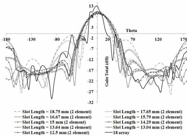
**Figure 10.** Plot of gain versus theta over  $\Theta = -180^\circ$  to  $180^\circ$  direction for the 18-element slot array and nine other two-element slot arrays corresponding to resonance frequencies 8, 8.5, 9, 9.5, 10, 10.5, 11, 11.5 and 12 GHz respectively.
