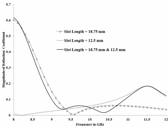
**Figure 5.** Variation of magnitude of reflection coefficients with frequency for three slot array antennas, one with non-uniform length (18.75 mm & 12.5 mm) and two with uniform lengths (18.75 mm & 12.5 mm respectively).
