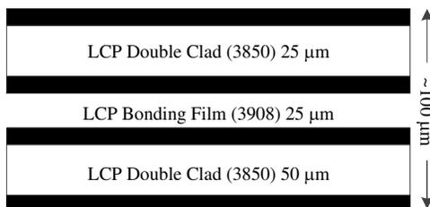
**Figure 2.** Multi-Layer configuration of the ultra-thin M-LCP process with overall thickness of  $100\ \mu\text{m}$ .
