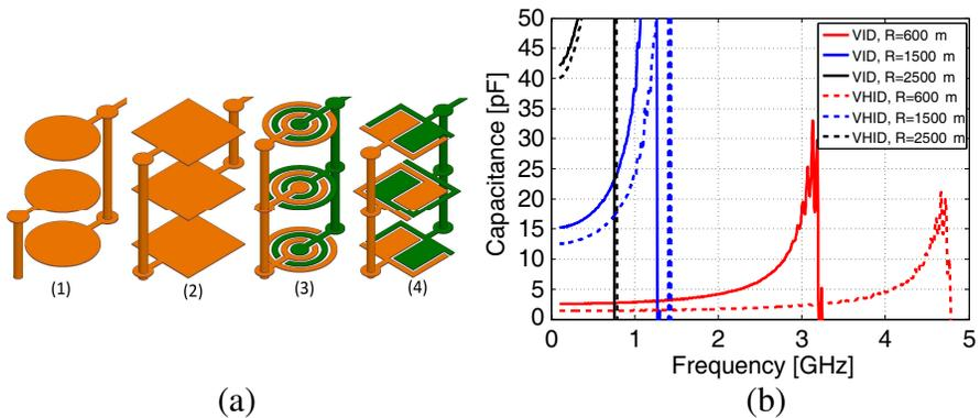
**Figure 6.** (a) 3D structures of LCP capacitors: (1) Circular VID capacitor. (2) Rectangular VID capacitor. (3) Circular VHID capacitor. (4) Rectangular VHID capacitors. (b) Measured capacitance of circular VID and VHID capacitors for various radii.
