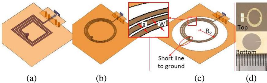
**Figure 3.** Spiral inductors. (a) Rectangular. (b) Circular with complete ground plane. (c) Circular with ground plane partially etched. (d) Photograph of the fabricated circular inductors with partially etched ground plane.
