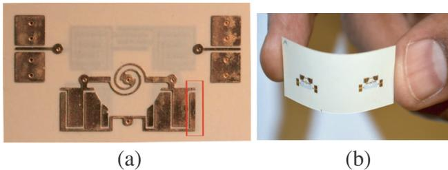
**Figure 8.** (a) A Photograph of the fabricated M-LCP bandpass filter. (b) Illustration of the flexibility of the LCP filter.
