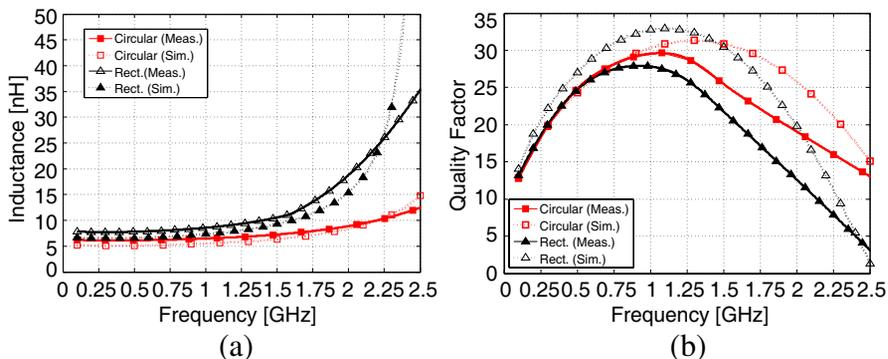
**Figure 4.** Comparison between circular and rectangular spiral inductors in terms of (a) Inductance, and (b)  $Q$  (smoothed using a standard MATLAB function which uses an average filter with local regression algorithm.).
