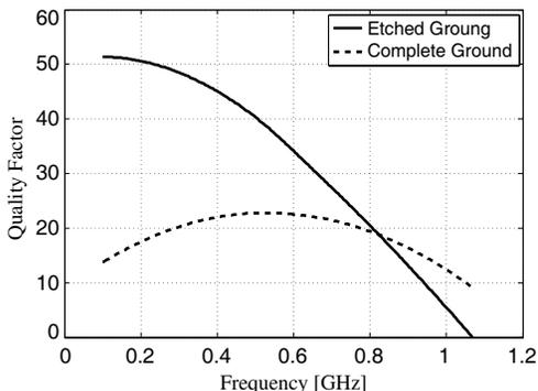
**Figure 5.** Measured  $Q$  (smoothed) of two different inductors (one with complete and the other with etched off ground as in Fig. 3). The inductor has  $N = 2.5$ ,  $R_o = 2500 \mu\text{m}$ , and  $s/W = 0.5$ .
