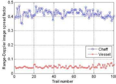
**Figure 4.** Range-Doppler image spread factors of the vessel and the chaff.
