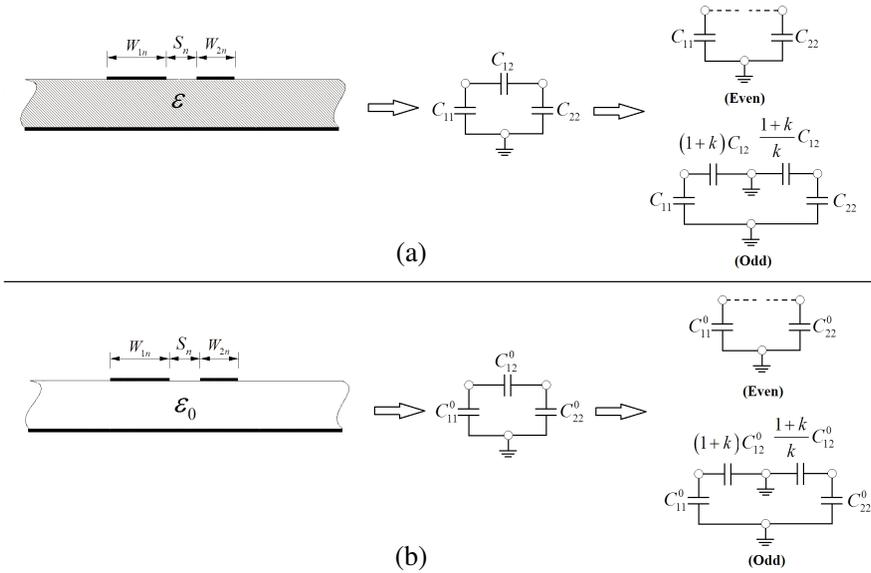
**Figure 2.** The cross section of uniform asymmetrical coupled lines over dielectric and vacuum substrates including equivalent capacitance networks.
