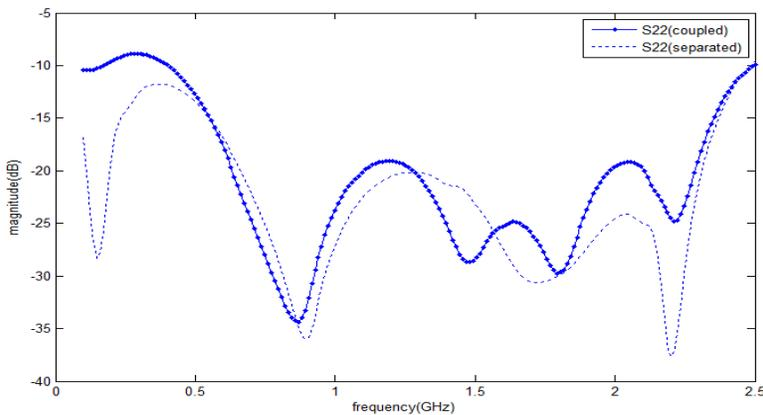
**Figure 9.** Reflection coefficient versus frequency at port 2.
