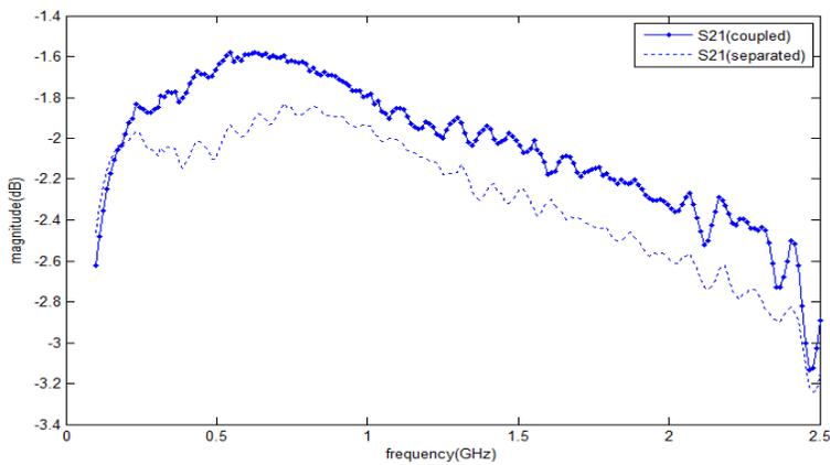
**Figure 6.** Measured power division versus frequency at port 2.
