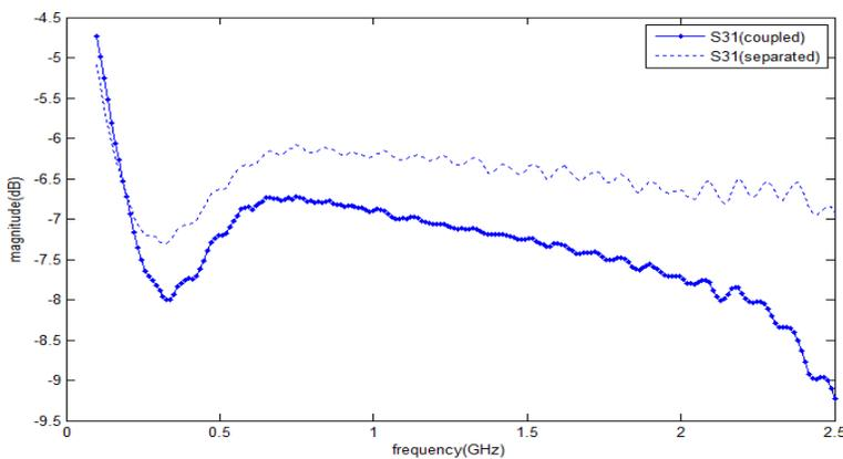
**Figure 7.** Measured power divisions versus frequency at port 3.
