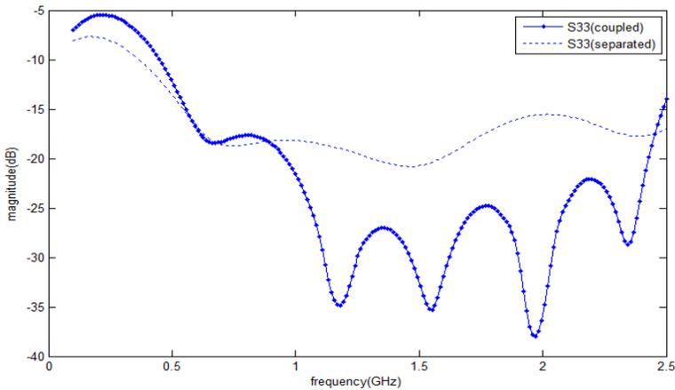
**Figure 10.** Reflection coefficient versus frequency at port 3.
