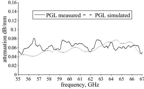
**Figure 14.** Measured and simulated attenuation of the PGL.
