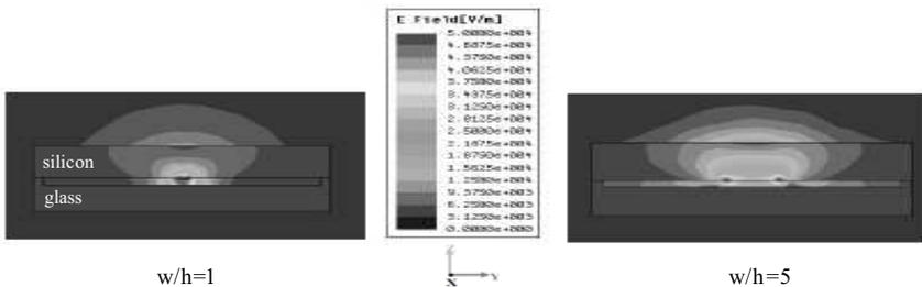
**Figure 9.** Electric field in magnitude in the transverse plane, for the IML ( $h = 100 \mu\text{m}$ ,  $H_{\text{silicon}} = H_{\text{glass}} = 500 \mu\text{m}$ ,  $t = 1 \mu\text{m}$ ) at 60 GHz for two  $W/h$  ratios ( $W/h = 1$  and 5).
