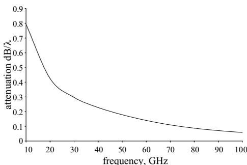
**Figure 5.** Attenuation ( $\text{dB}/\lambda$ ) of the IML versus the frequency ( $h = 100 \mu\text{m}$ ,  $W = 100 \mu\text{m}$ ,  $t = 1 \mu\text{m}$ ) at 60 GHz.
