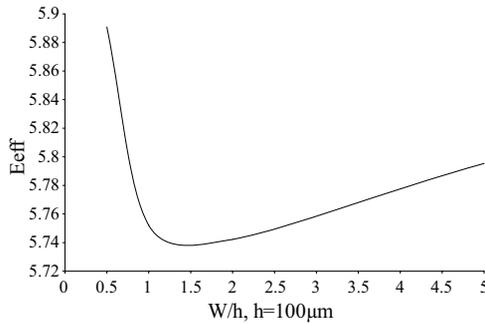
**Figure 8.** Effective permittivity for the IML ( $h = 100 \mu\text{m}$ ,  $H_{\text{silicon}} = H_{\text{glass}} = 500 \mu\text{m}$ ,  $t = 1 \mu\text{m}$ ) versus different  $W/h$  ratio ( $W/h$  from 0.5 to 5) at 60 GHz.
