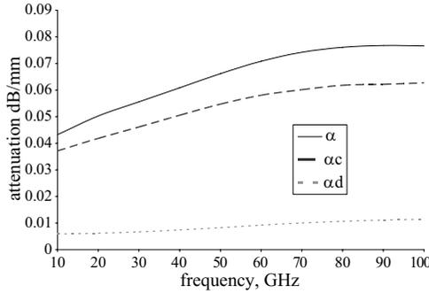
**Figure 7.** Attenuation (dB/mm) of the IML versus frequency (10–100 GHz) ( $t_{strip} = 1 \mu\text{m}$ ;  $H_{silicon} = 500 \mu\text{m}$ ;  $W = 100 \mu\text{m}$ ;  $h = 100 \mu\text{m}$ ) in considering total losses  $\alpha$ , metallic losses  $\alpha_c$  or dielectric losses  $\alpha_d$ .
