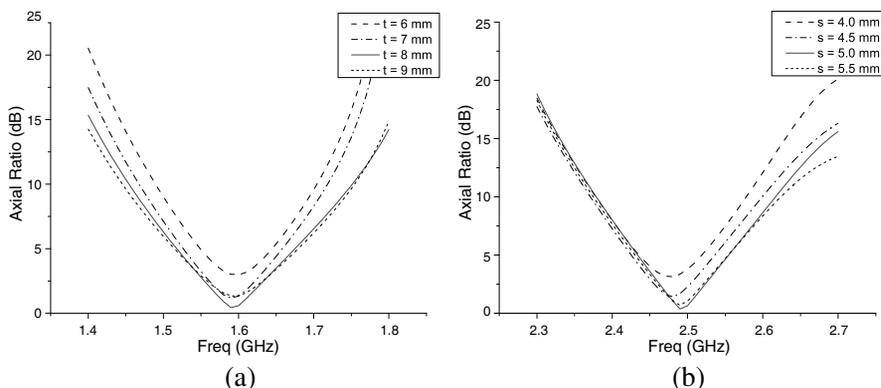
**Figure 9.** Axial ratio against frequency of Antenna-2 (a) at lower band for various  $t$  and (b) at upper band for various  $s$ .
