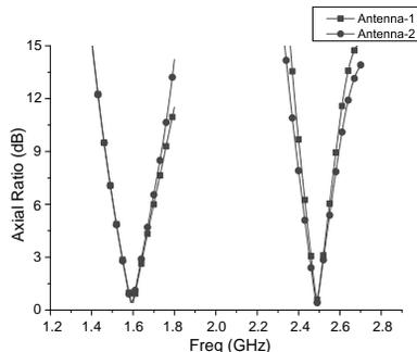
Figure 4. Axial ratio of the two antennas.
