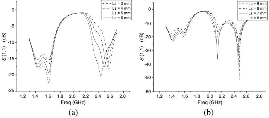
**Figure 7.** Return loss against frequency of the proposed (a) Antenna-1 and (b) Antenna-2 for various  $L_s$ .
