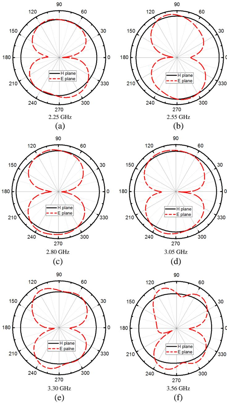
**Figure 13.** The measured radiation pattern of each frequency.
