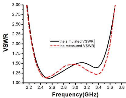
**Figure 11.** The measured VSWR of the proposed antenna.
