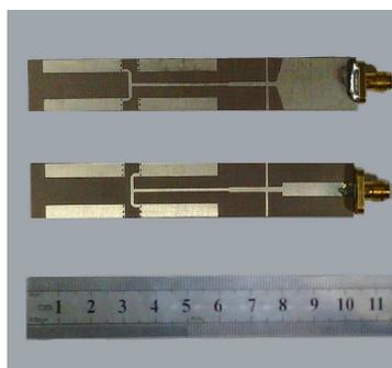
**Figure 12.** The top view of the proposed antenna.
