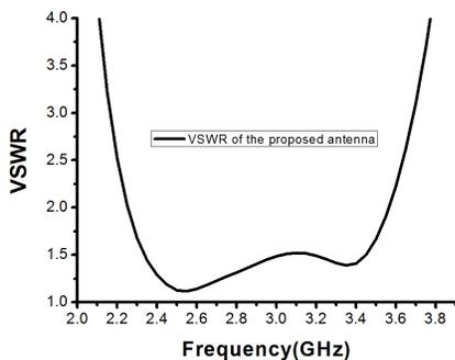
**Figure 10.** The VSWR of the proposed antenna.
