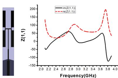
Figure 7. The input impedance of the antenna with balun.
