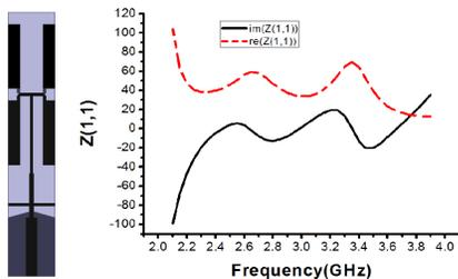
Figure 8. The input impedance of the proposed antenna.
