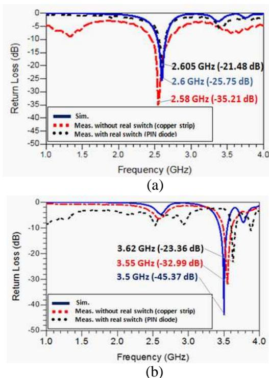
**Figure 14.** Comparison of  $S_{11}$  values between simulated and measured results during (a) ON mode and (b) OFF mode.
