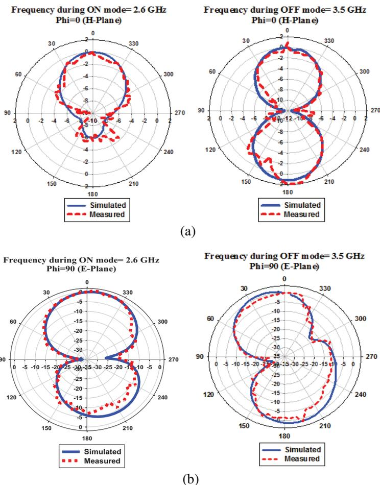
**Figure 12.** Simulated and measured radiation patterns in polar plot during ON mode at 2.6 GHz and OFF mode at 3.5 GHz with (a)  $\Phi = 0$  ( $H$ -plane) and (b)  $\Phi = 90$  ( $E$ -plane).
