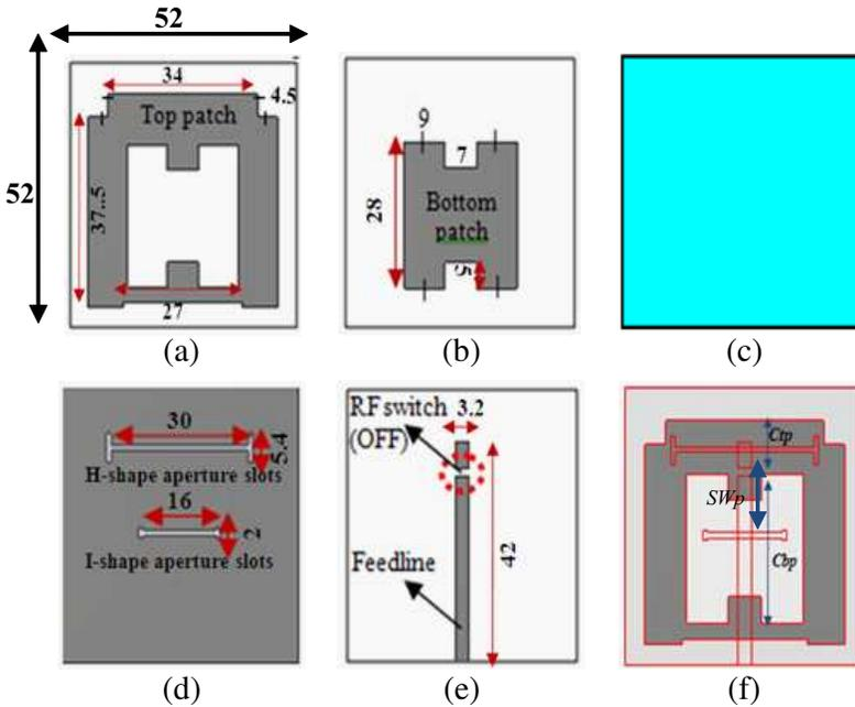
**Figure 2.** Geometry and dimensions (mm) of the FRSPMA. (a) Substrate 1: Top patch, (b) substrate 2: Bottom patch, (c) air-filled gap, (d) ground plane with two aperture slots, (e) substrate 3: Feed network with one RF switch (back view), and (f) geometry of the whole antenna structure in 1-plane view.
