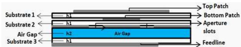
Figure 1. Side view structure of the FRSPMA.
