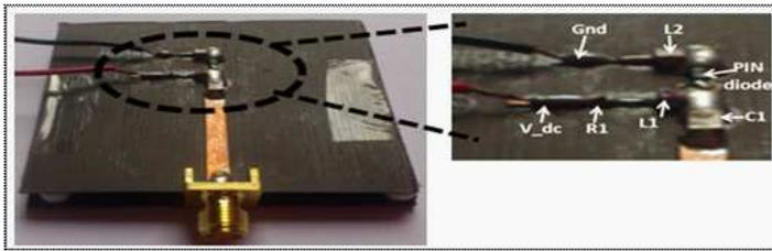
**Figure 5.** The back view of the FRSPMA with equivalent switching circuit models.
