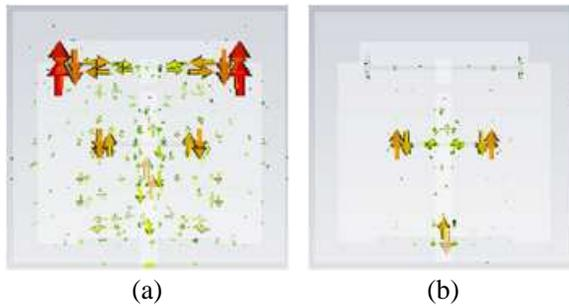
**Figure 9.** Simulated results of surface current from back view of the FRSPMA during (a) ON mode at 2.6 GHz and (b) OFF mode at 3.5 GHz.
