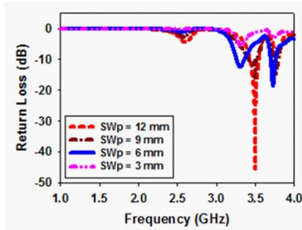
**Figure 8.** The return loss effects of switch position along  $SW_p$  during SW OFF.
