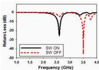
**Figure 10.** Simulated results of return loss when the switch is in ON and OFF modes.
